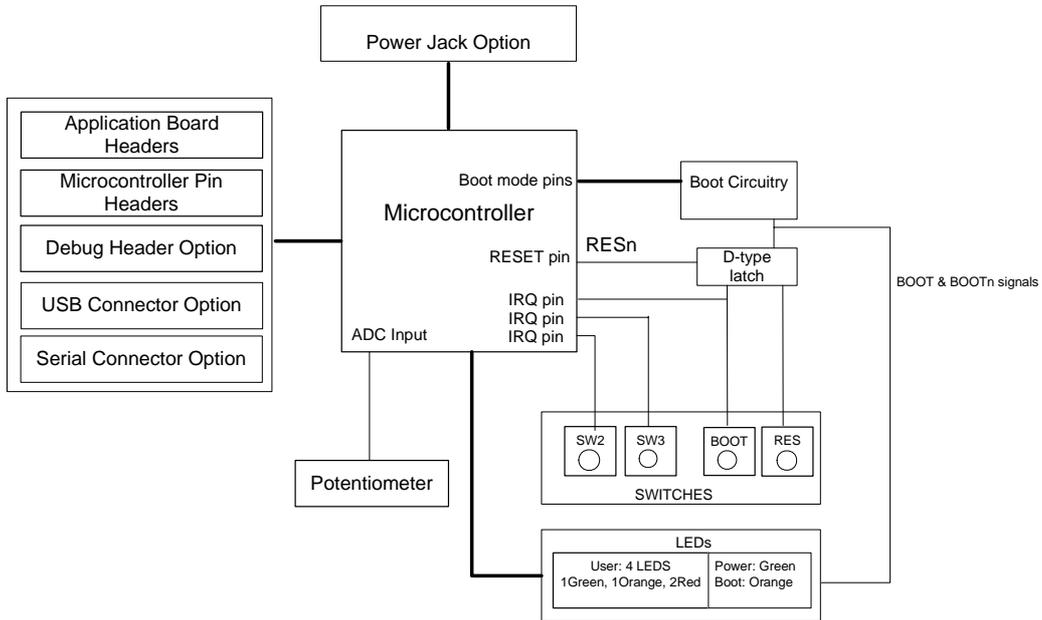
Figure 5.1: Block Diagram
