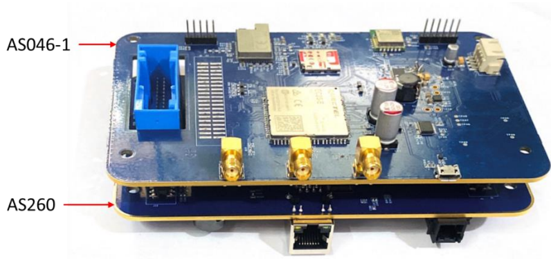
Figure 4-10 AS049-1-REIN-WCU-V1 and AS260 stack up.
