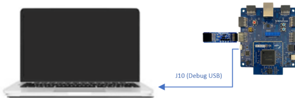
Figure 16. Connecting the AIK-RA6M3 Board to the Host PC via USB Debug Port
