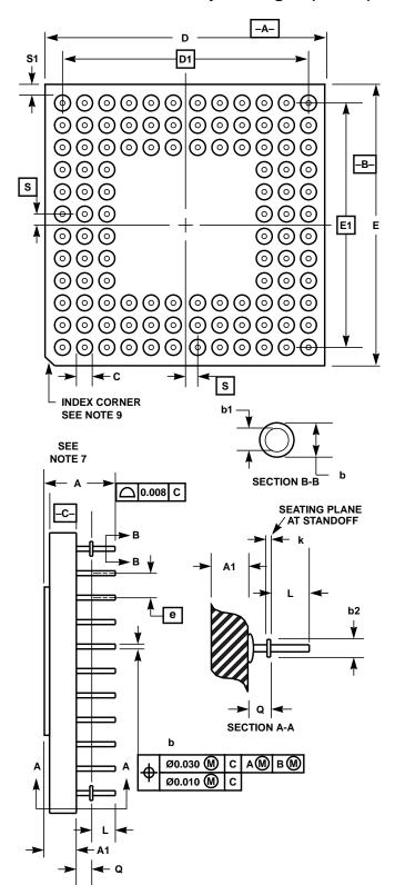
**G68.A** MIL-STD-1835 CMGA3-P68C (P-AC) 68 LEAD CERAMIC PIN GRID ARRAY PACKAGE
