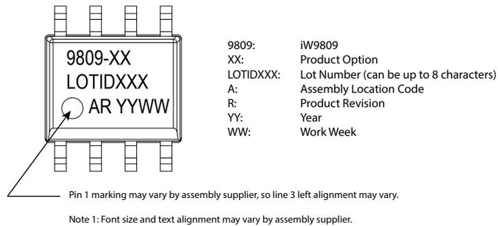
**Figure 8.1 : Top Marking for the iW9809**
