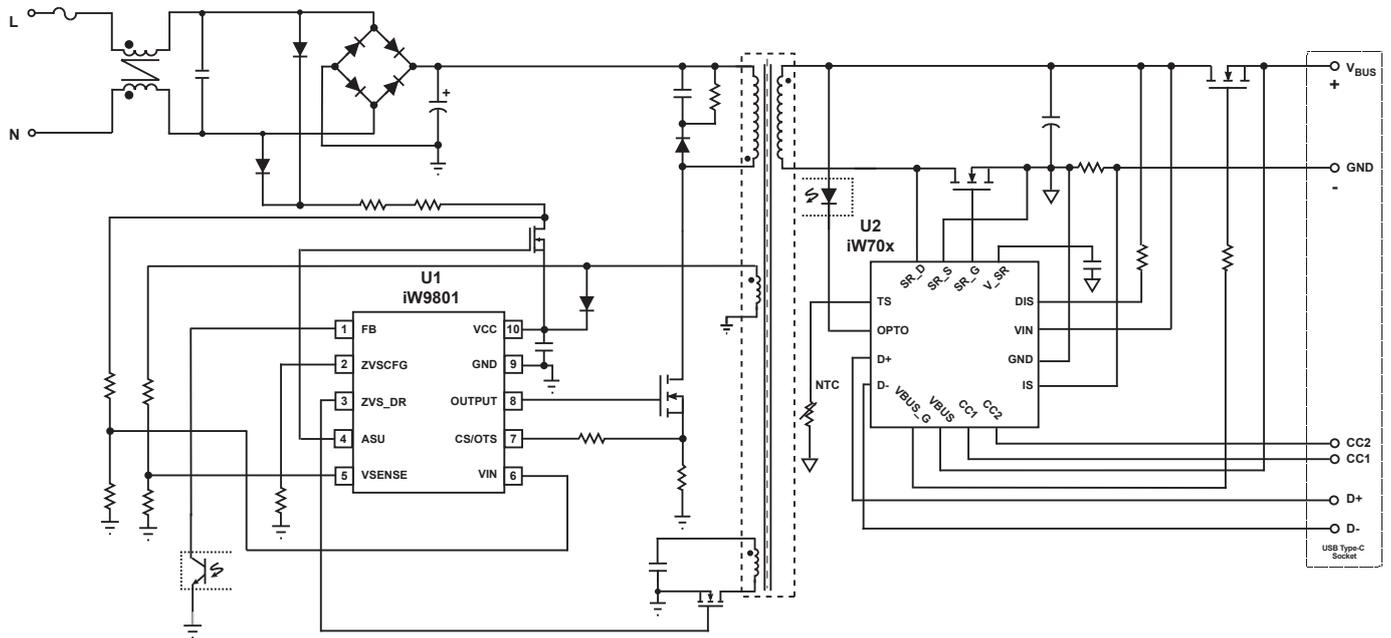
Figure 3.1 : iW9801 Typical Application Circuit with Active Start-up Circuit
