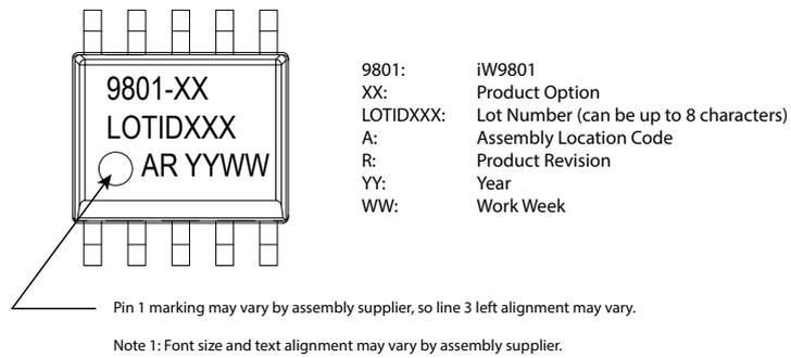
Figure 8.1 : Top Marking for the iW9801 (SOIC-10)
