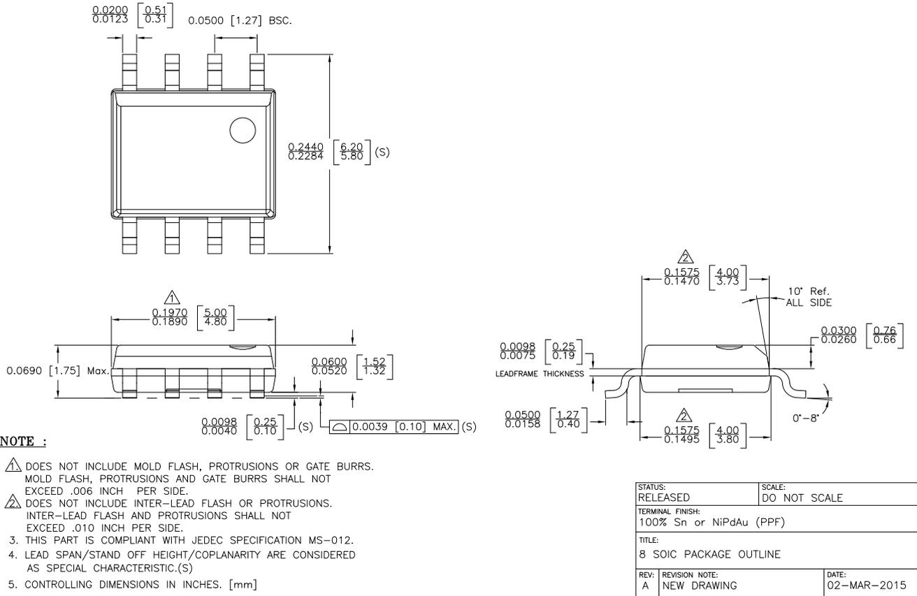
Figure 6.1 : Physical Dimensions of 8-Pin SOIC Package
