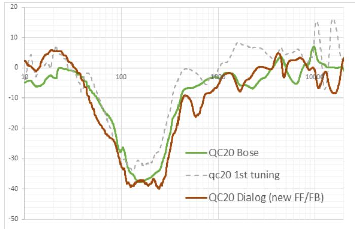
Key to this performance is a custom DSP that is optimized for ANC and enables an input-to-output latency of just 25  $\mu$ s. Meanwhile a dedicated fast equalization (FEQ) path operating at the digital microphone (DMIC) clock rate improves cancellation at high frequencies.
