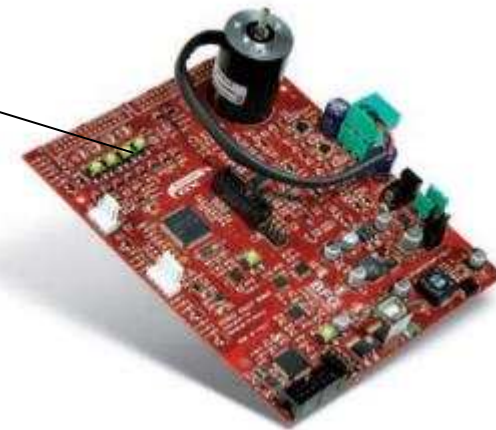
Single PCB inverter based on RX62T + AC Brushless motor
