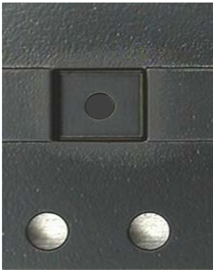
Existing Carrier Tape- Pocket Design
