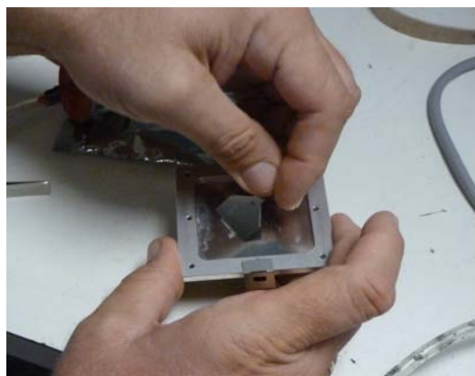
FIGURE 17. DEPOSIT PASTE WITH SMALL SQUEEGEE BLADE
