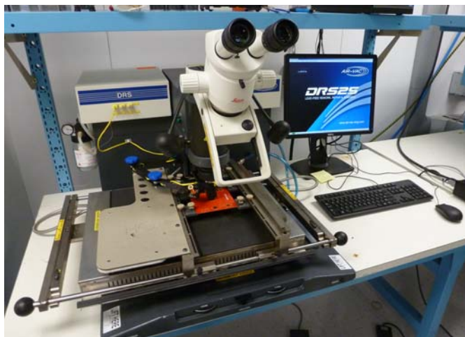
FIGURE 8. REWORK STATION WITH THERMAL PROFILE CONTROL
