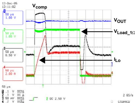
FIGURE 2. TRANSIENT RESPONSE AT 7V V<sub>IN</sub>
