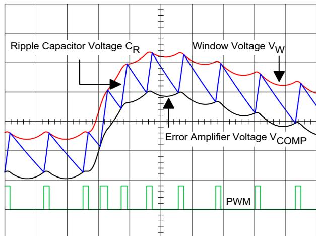
FIGURE 1. MODULATOR LOAD TRANSIENT WAVEFORMS
