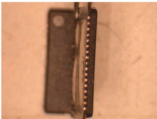
Figure 17. Finished Tinned Thermal Land on QFN
