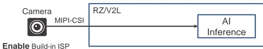
Camera signal pipeline after applied RZ/V2L ISP Support Package
