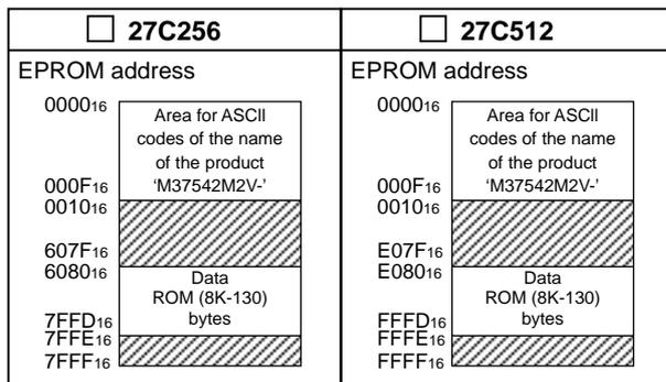
In the address space of the microcomputer, the internal ROM area is from address E080<sub>16</sub> to FFFD<sub>16</sub>. The reset vector is stored in addresses FFFC<sub>16</sub> and FFFD<sub>16</sub>.
