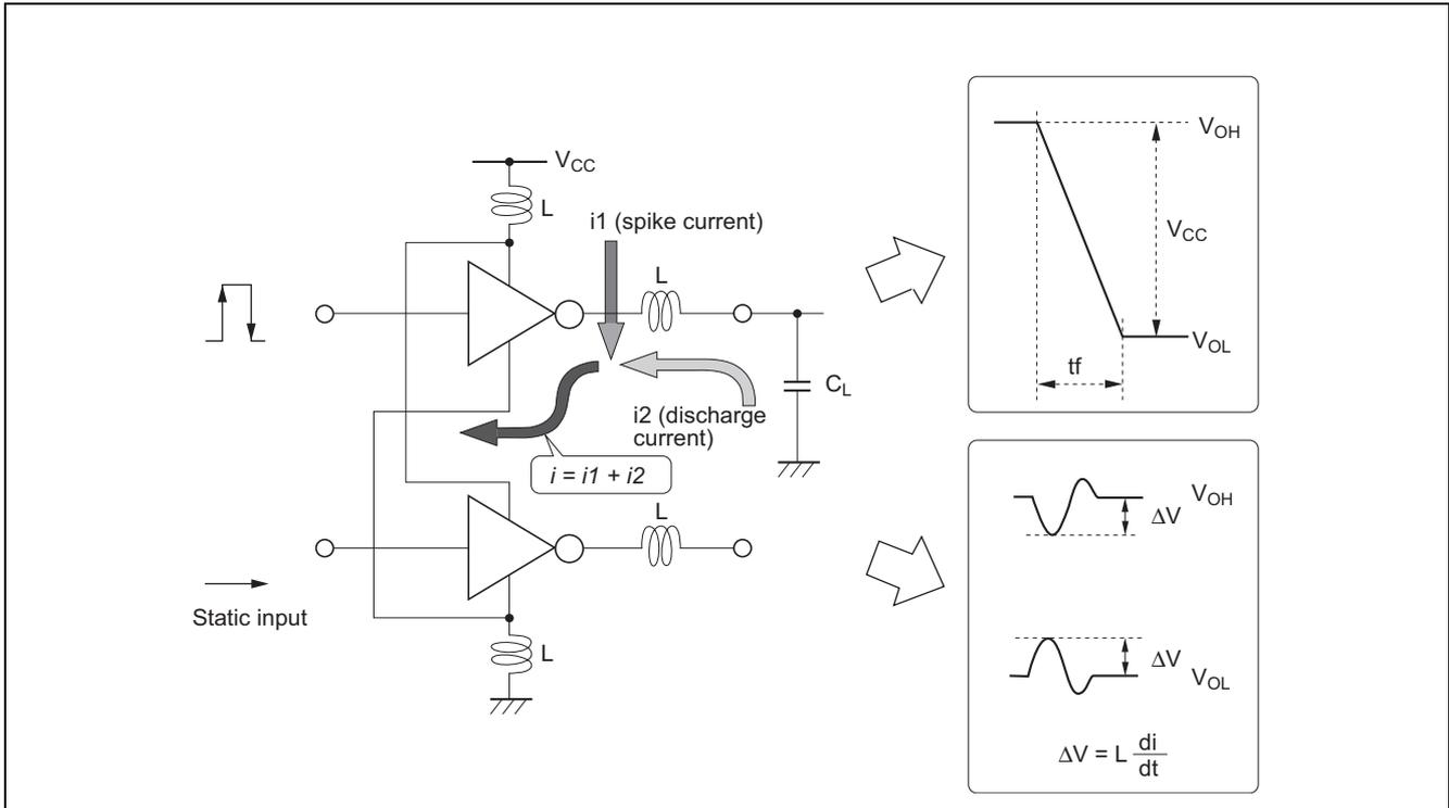
Figure 5-12 Principle of Simultaneous Switching Noise
