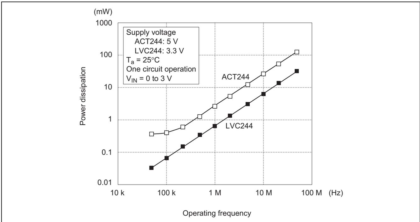
Figure 4-11 Power Dissipation in Relation to Operating Frequency
