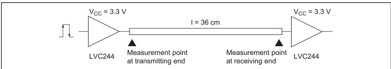
Figure 5-1 Noise Test Circuit
