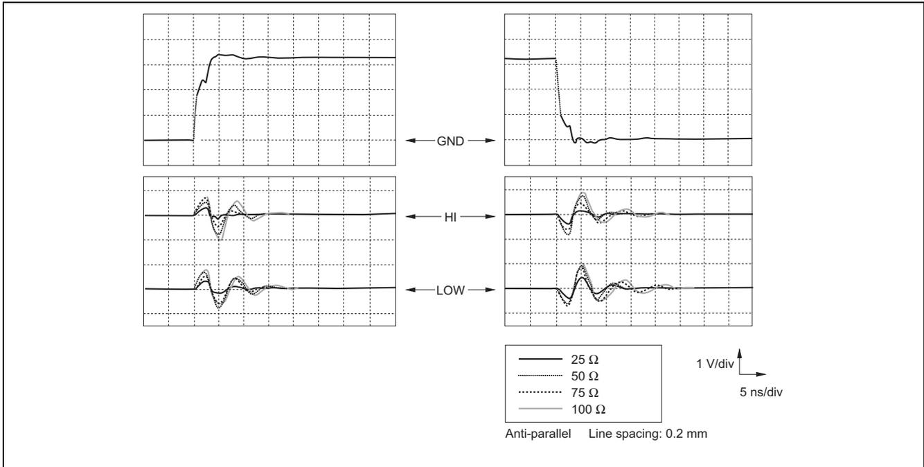
**Figure 5-11-3 Crosstalk (Effect of Effect of Transmission Line Impedance)**
