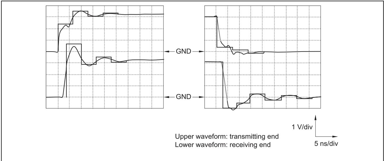
Figure 5-5-3 Analysis of Reflection Waveforms (Comparison with Actual Waveforms)
