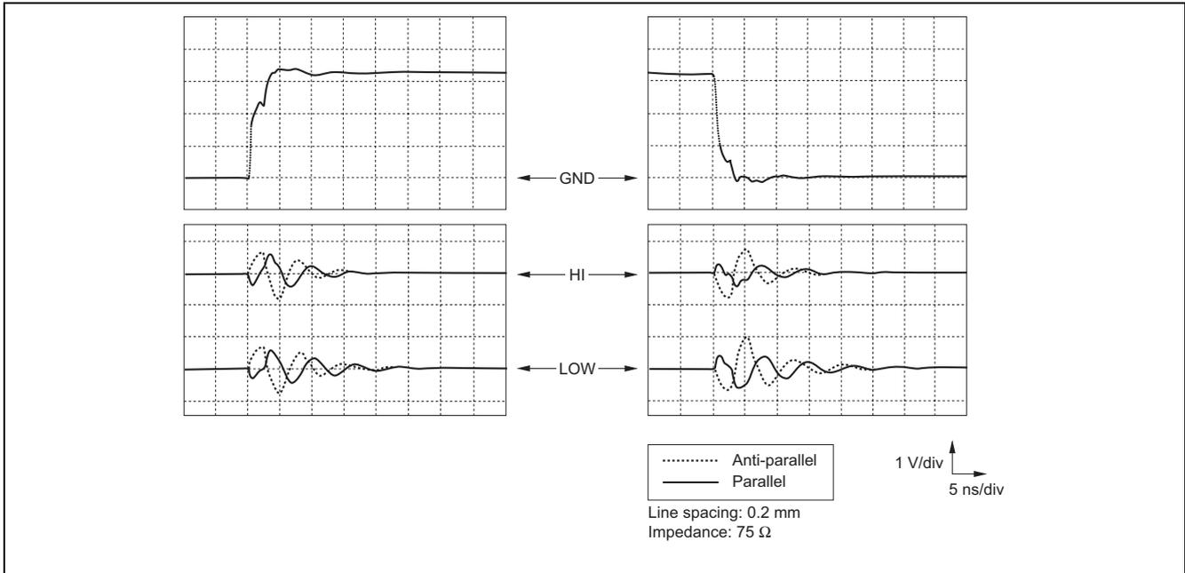
Figure 5-11-1 Crosstalk (Comparison of Parallel and Anti-Parallel Cases)
