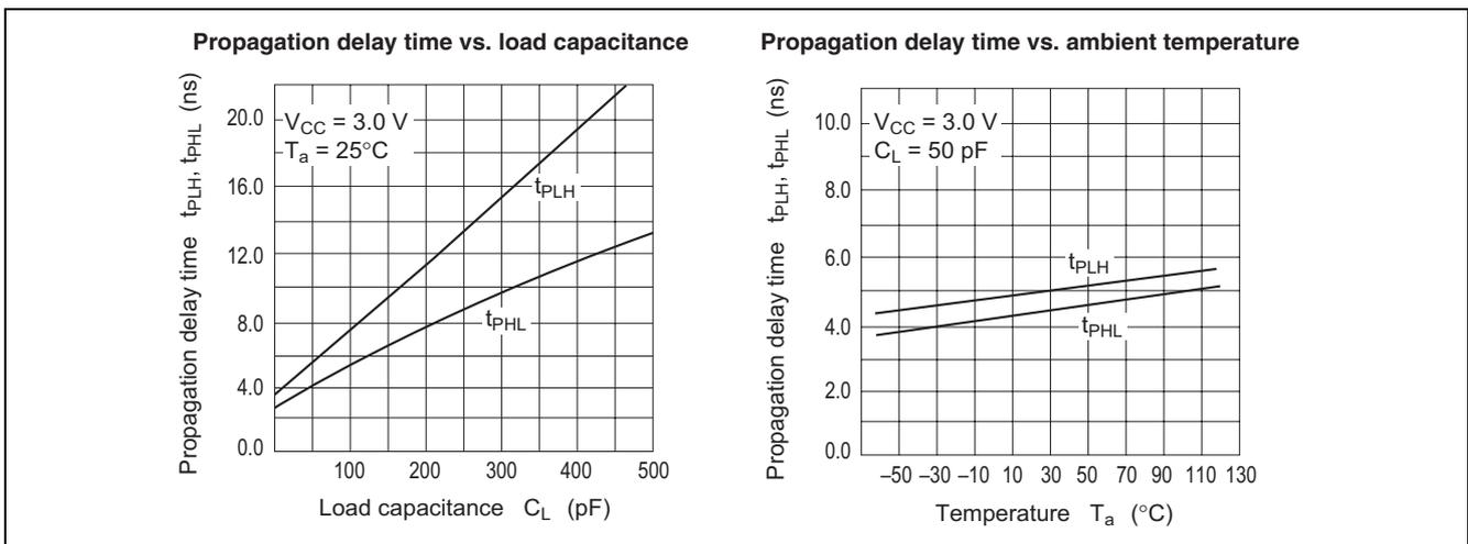
Figure 4-10 Measured Propagation Delay Time
