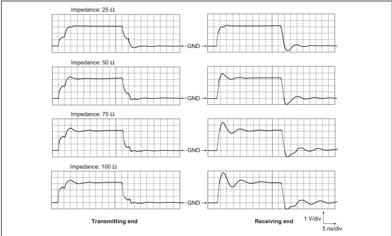
**Figure 5-7 Reflection Noise Waveforms**
