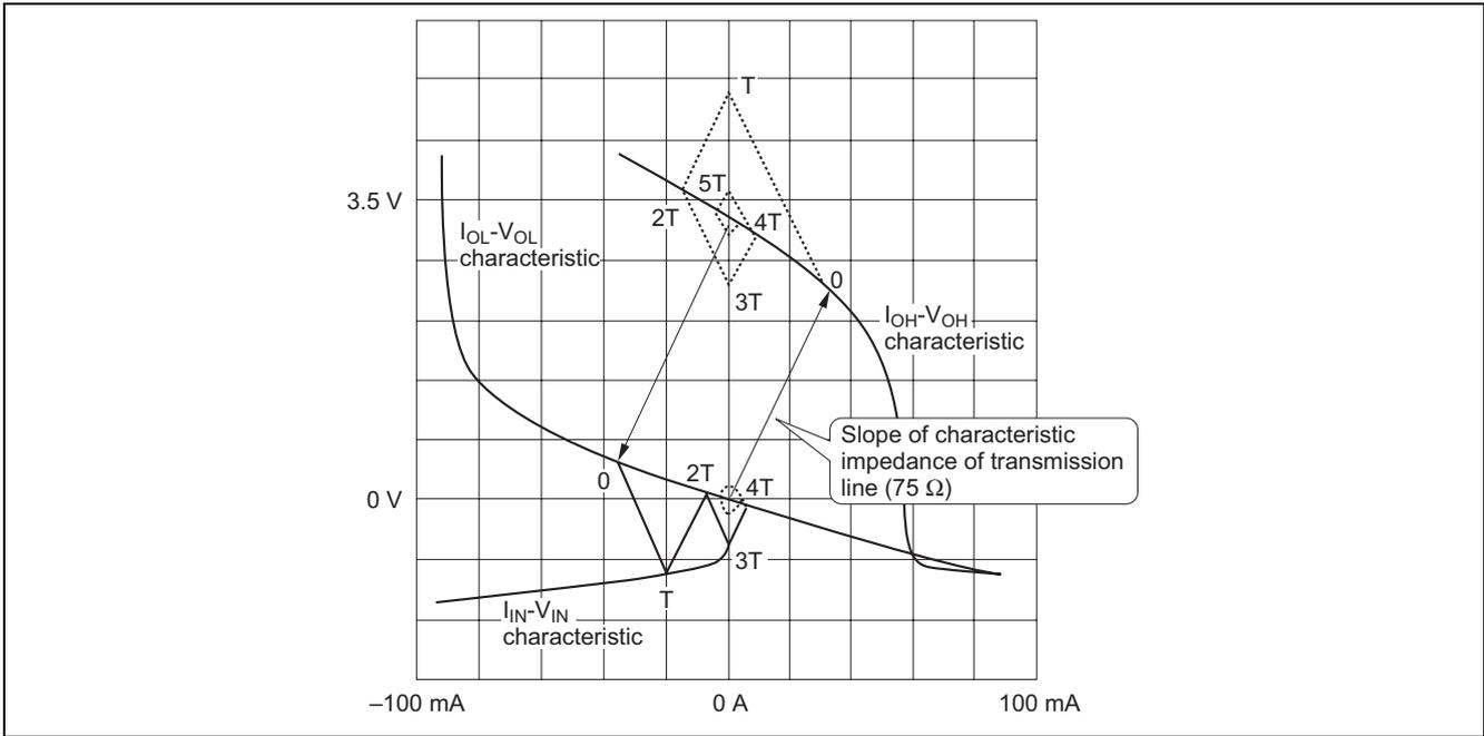
Figure 5-5-1 Analysis of Reflection Waveforms (Bergeron Diagram)
