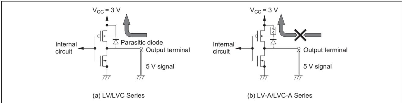
**Figure 4-3 LVC-A and LV-A Series Output Circuit**
