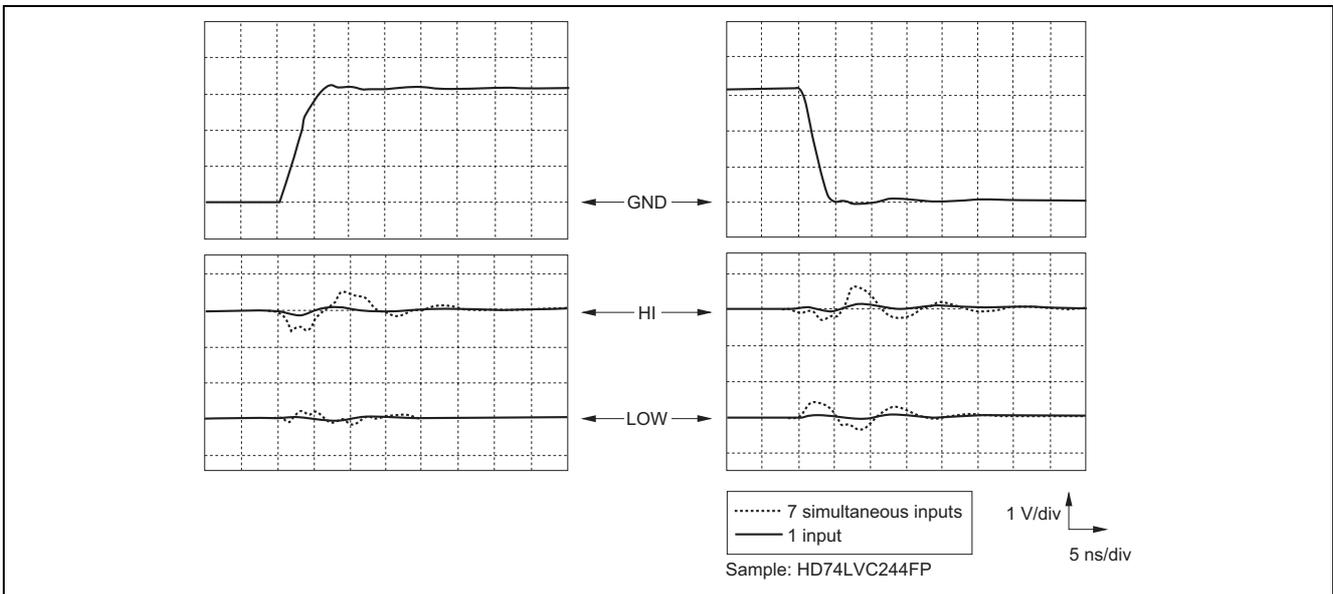
Figure 5-14-1 Multiple Output Switching Noise
