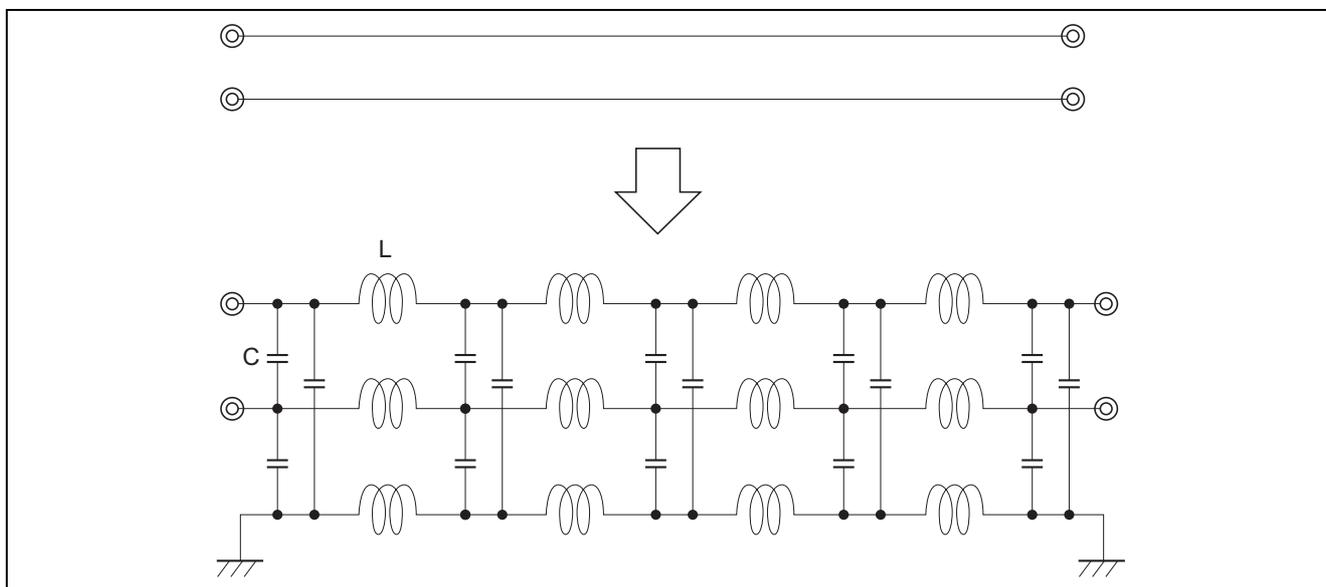
Figure 5-3 Conceptual Diagram of Transmission Lines
