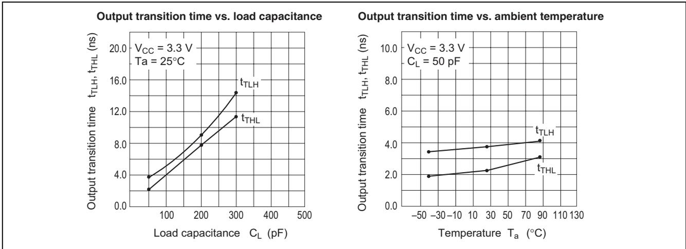
Figure 4-9 Measured Output Transition Time
