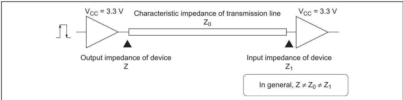
Figure 5-4 Reflection Principle
