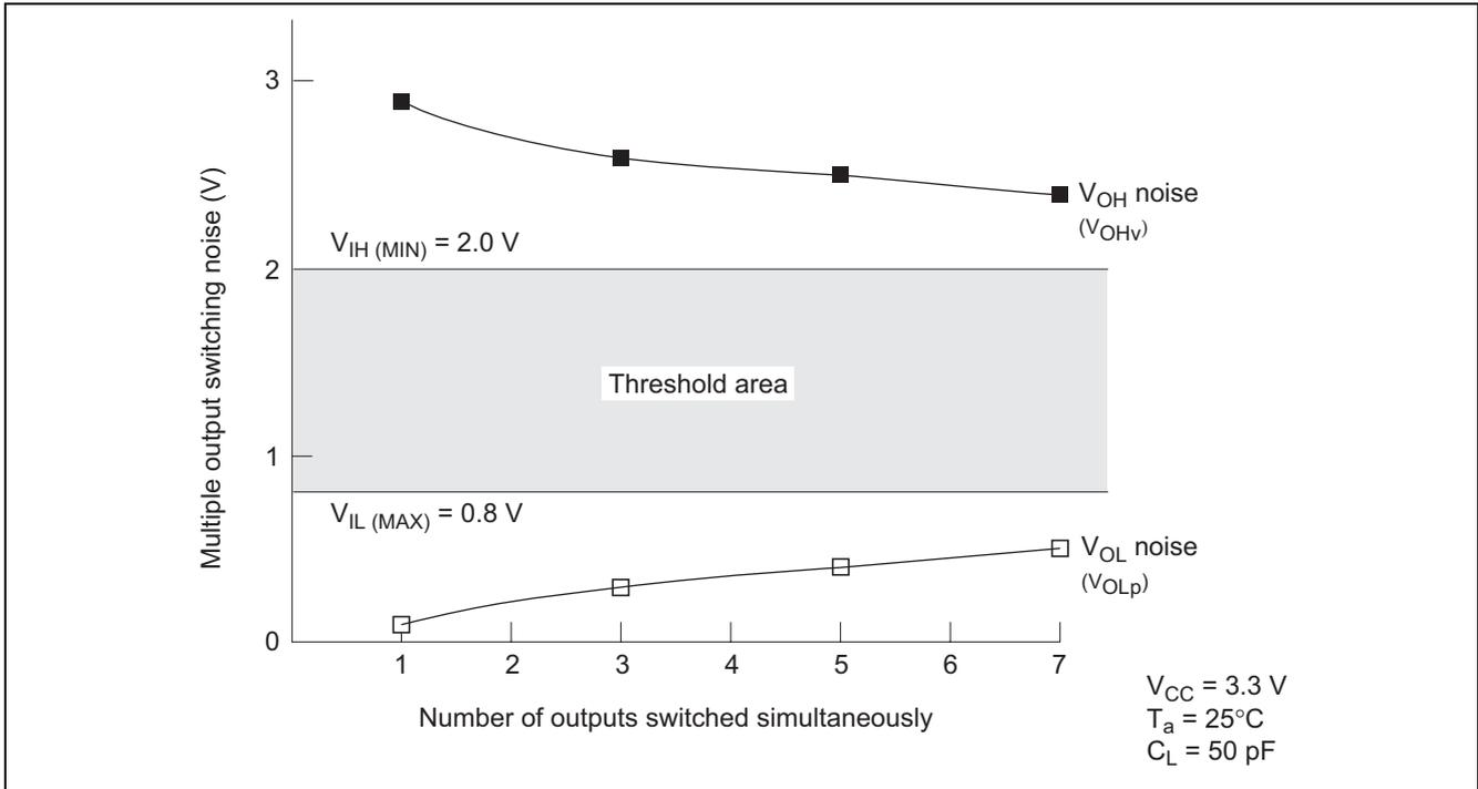
Figure 5-15 Effect of Number of Simultaneously-Switched Circuits
