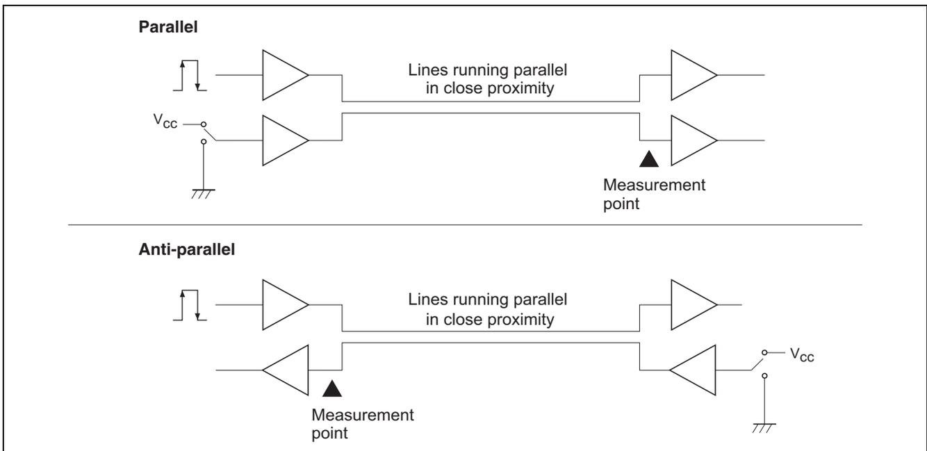
Figure 5-10 Circuits for Measuring Crosstalk Noise
