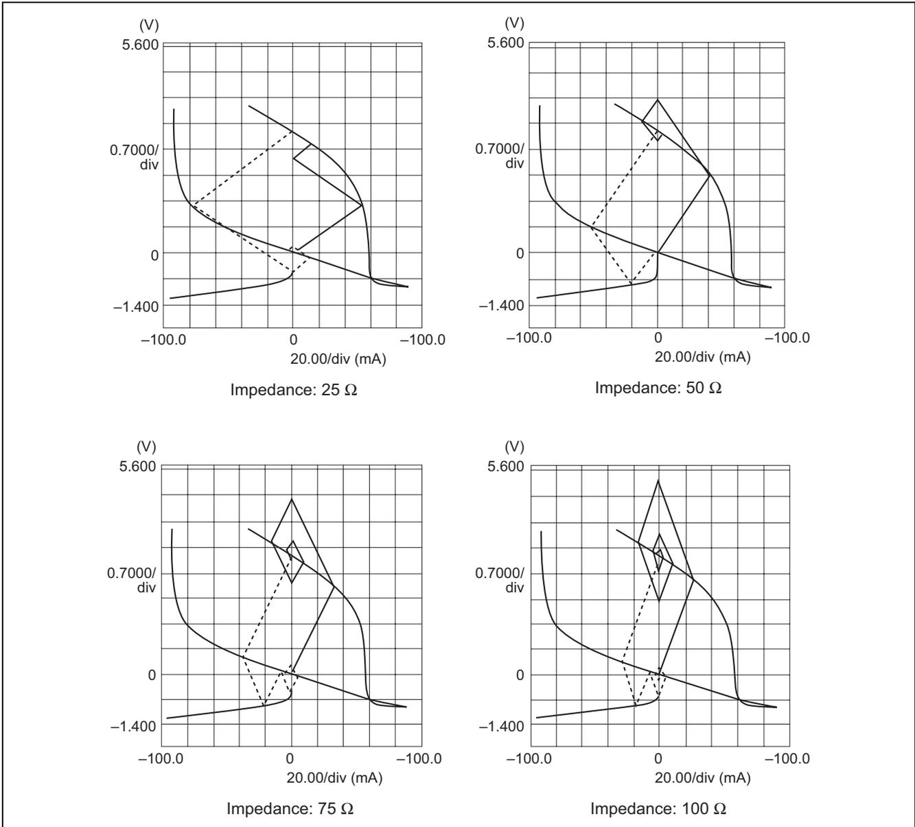
Figure 5-6 Reflection Waveform Analysis for Various Circuits
