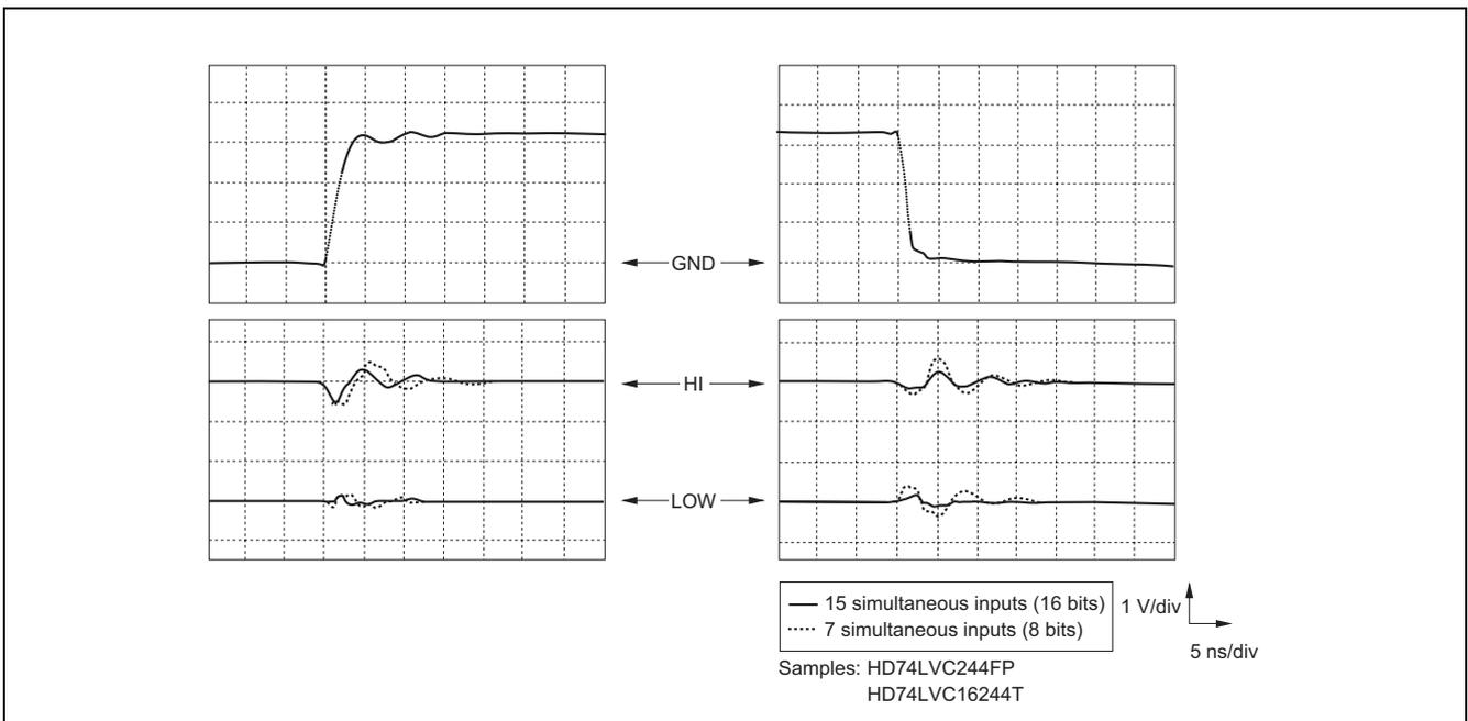
**Figure 5-14-3 Multiple Output Switching Noise (Comparison of 8-Circuit and 16-Circuit Packages)**
