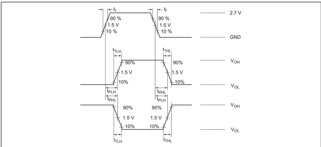
Figure 4-8 Measured Waveform Parameters and Symbols
