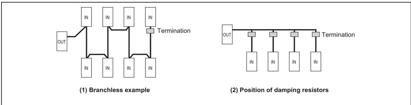
**Figure 5-8 Examples of Termination**
