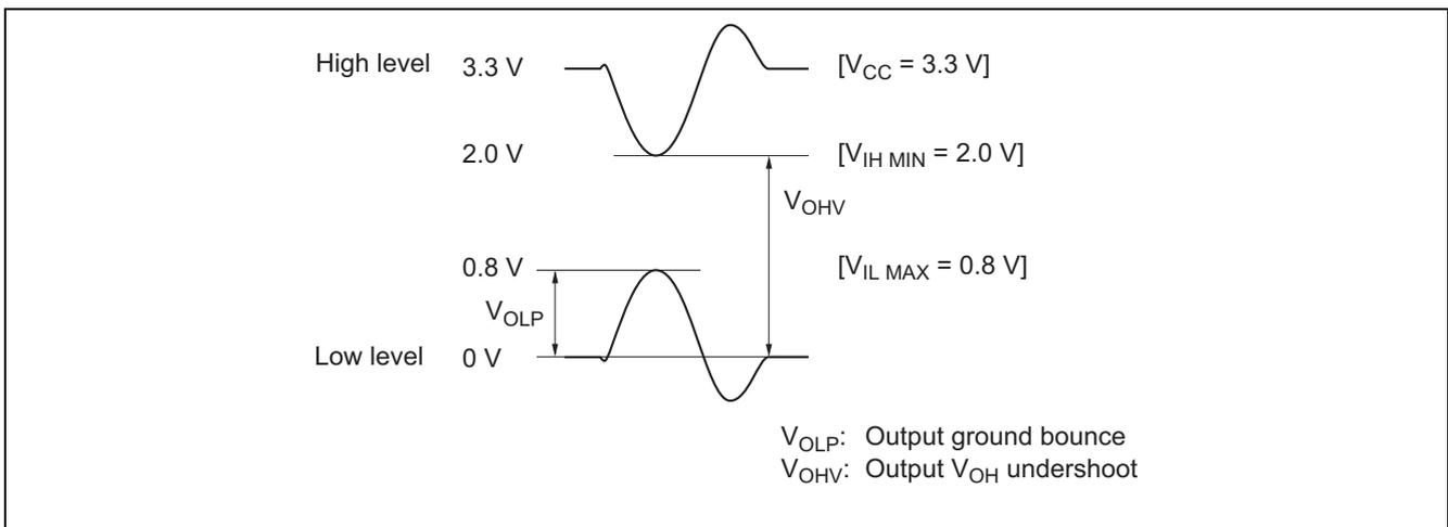
**Figure 3-1 Output Noise Waveforms and Symbols**
