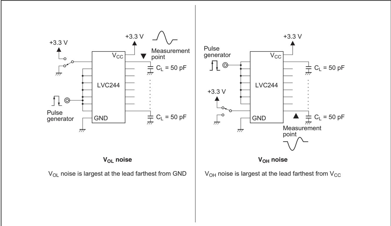
Figure 5-13 Circuits for Measurement of Simultaneous-Switching Noise
