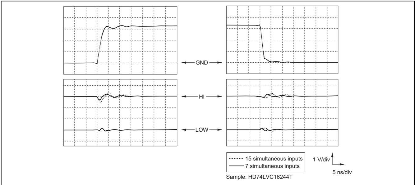
**Figure 5-14-2 Multiple Output Switching Noise
