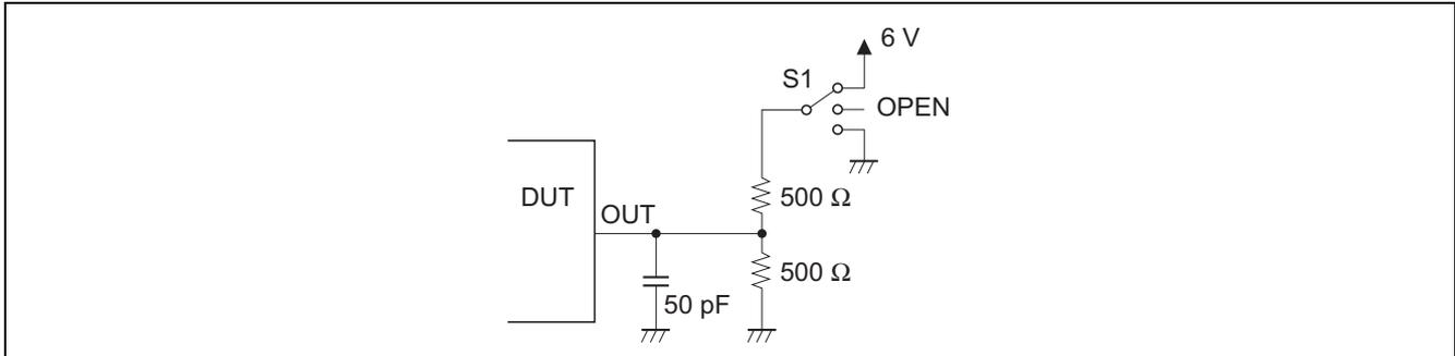
Figure 4-7 Test Circuit for AC Characteristics
