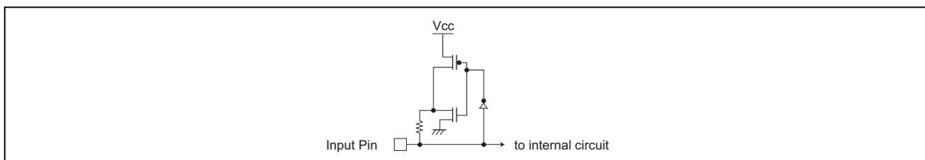
Figure 6-1 Bus hold Circuit
