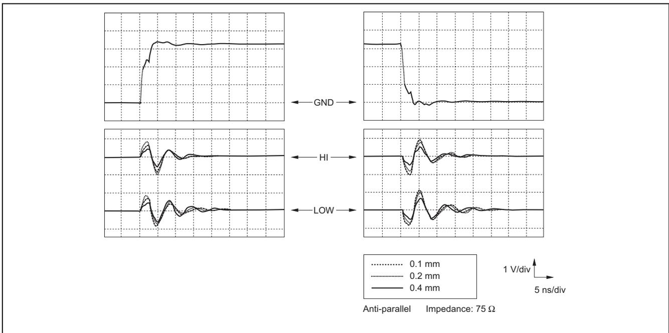
Figure 5-11-2 Crosstalk (Effect of Line Spacing)
