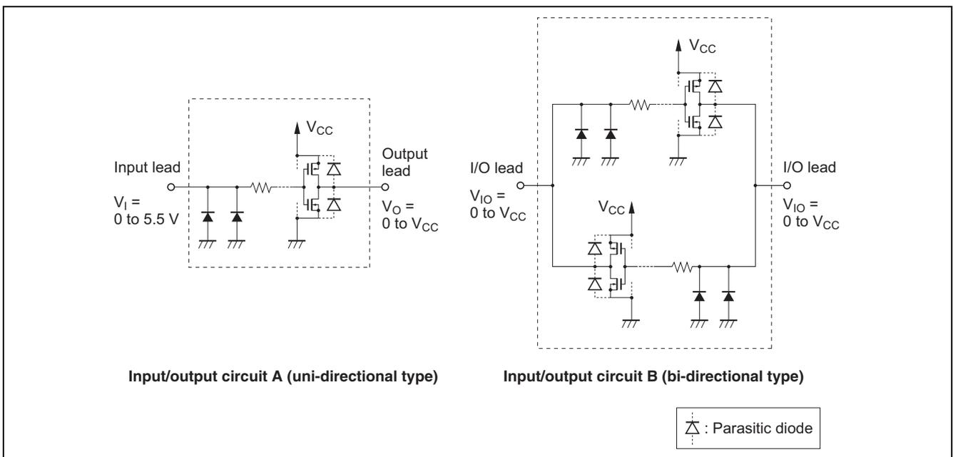
Figure 4-2 LV-A and LVC Series Input/Output Circuits
