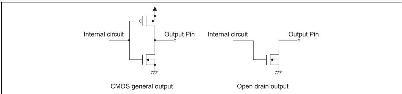
**Figure 4-5 The difference in output structure between general CMOS and open drain**
