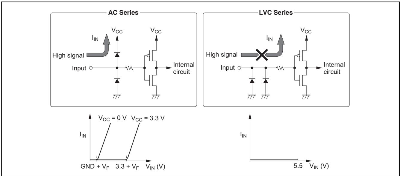
Figure 4-1 Input Protection Circuits of LV-A and LVC/LVC-A Series (Prevention of Current Leakage)
