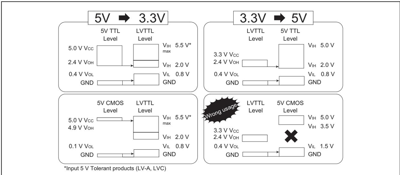
**Figure 4-4 Comparison of 3.3-V and 5-V Voltage Levels**
