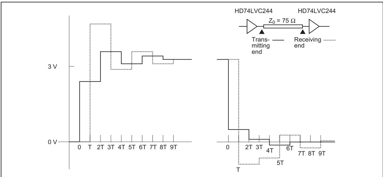
Figure 5-5-2 Analysis of Reflection Waveforms (Theoretical Waveform Plot)
