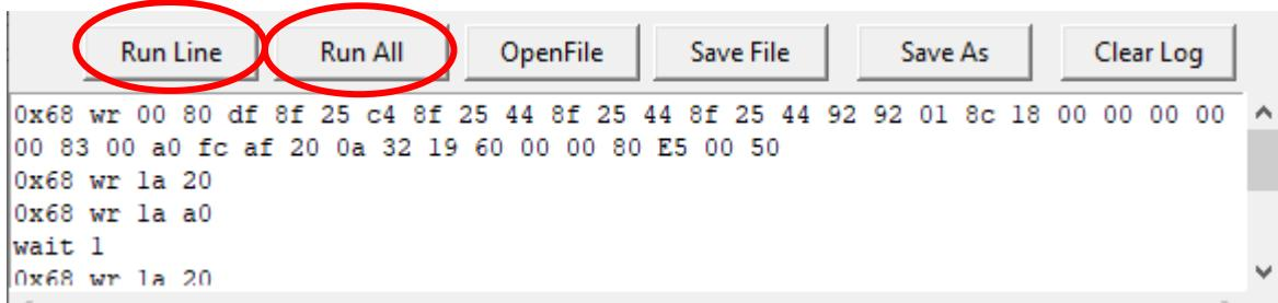
**Run Line:** This will execute the command line where the cursor is located. After the execution, the cursor will move to the next line.
