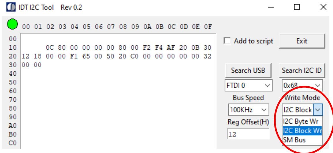
**I2C Byte Write mode:** This will write one byte at a time. Register offset address will increment for each write. The following is the example for the above picture data in byte write:
