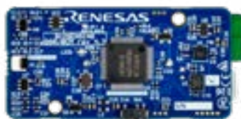
Biosensing GSR/BCM Reference Design
