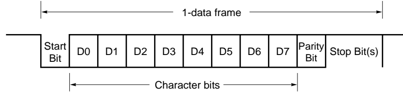
Figure 19-5. Asynchronous Serial Interface Transmit/Receive Data Format
