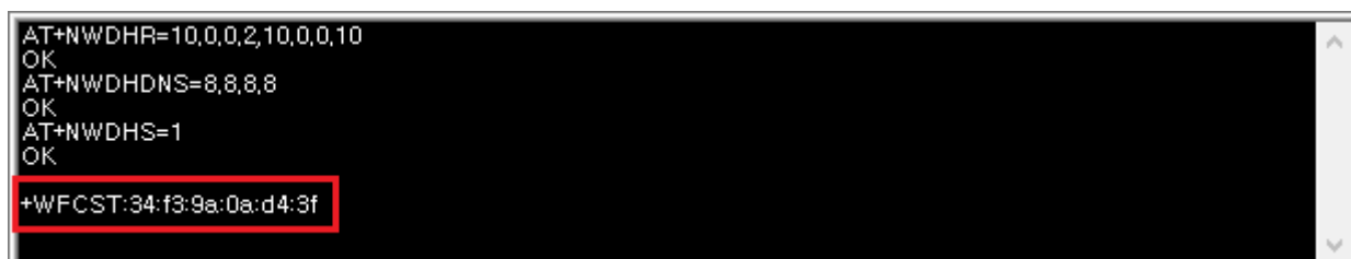
Figure 23. Debug console – DHCP configuration
