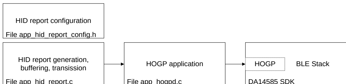
Figure 13: HID Report Module Block Diagram
