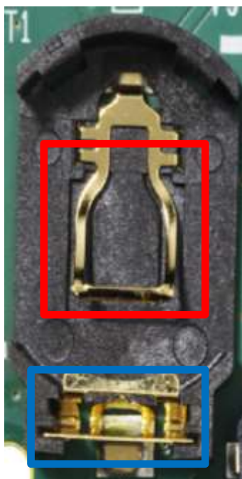
Figure 17: Removing the coin cell battery
