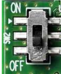
Figure 11: The actual Power supply switch (SW2)
