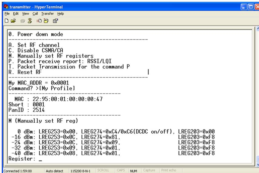
Figure 42: RF-Test Output power adjustment 1
