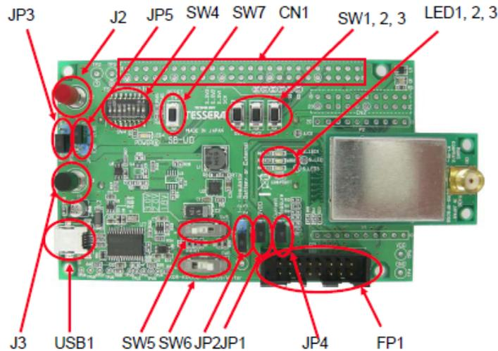
Figure 1: TK-RF8058+SB-EE demonstration board (Top View)
