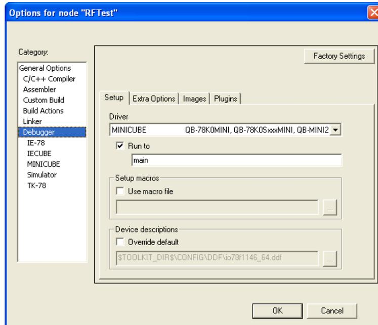
Figure 32: IAR Embedded Workbench Debugger Settings
