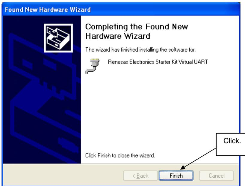
Figure 19: USB Driver Installation Completion (Windows XP)
