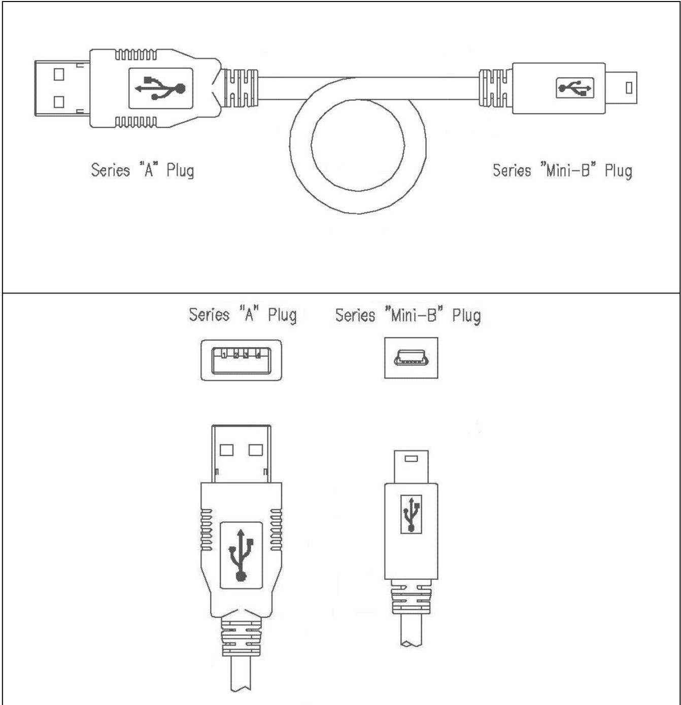
Figure 44: USB interface cable (Mini-B type)
