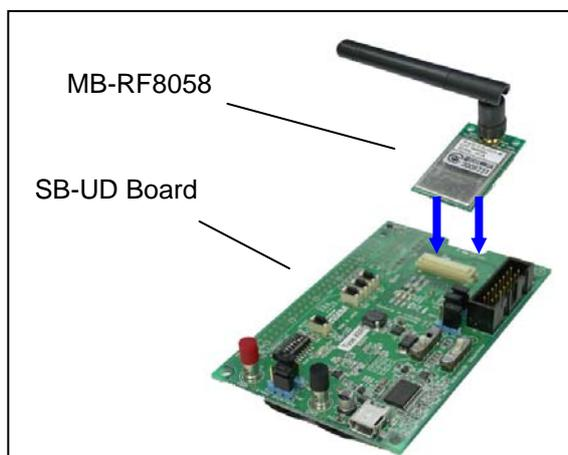
Figure 3: Mount MB-RF8058 to SB-UB
