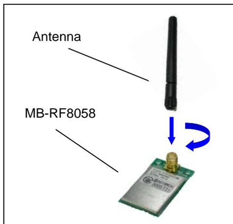
Figure 2: Mount antenna to MB-RF8058
