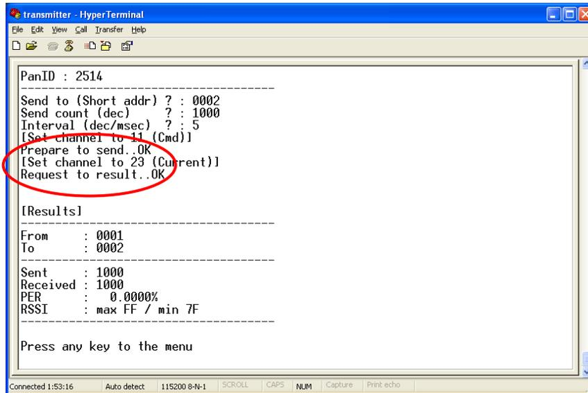
Figure 41: RF-Test PER test Channel 23
