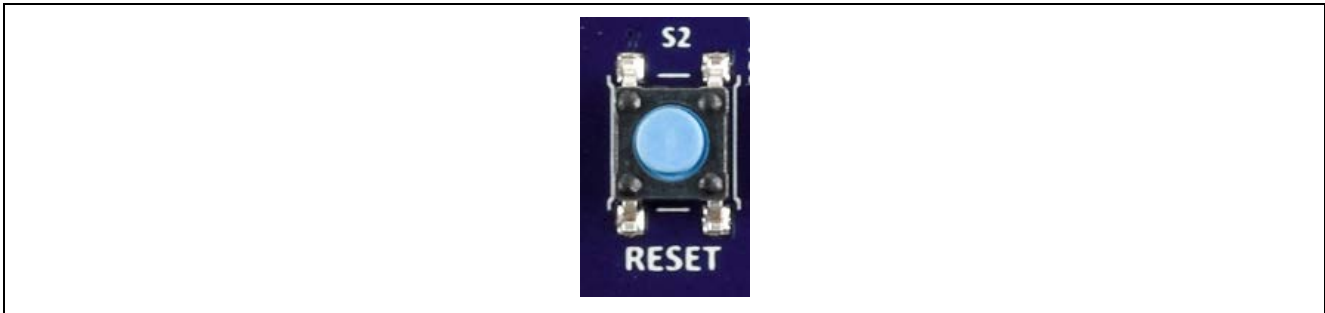
Figure 19. Reset Switch (S2) on the Target Board
