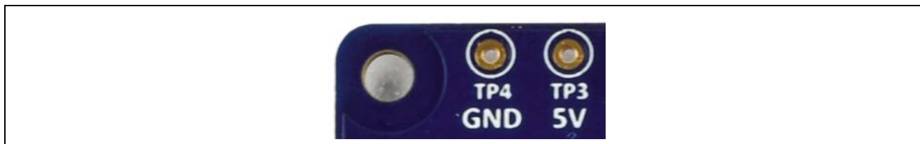
Figure 7. TP3 and TP4 on the Target Board
