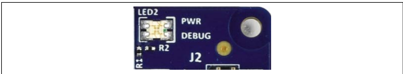
Figure 11. LED2 on the Target Board (Top Side)
