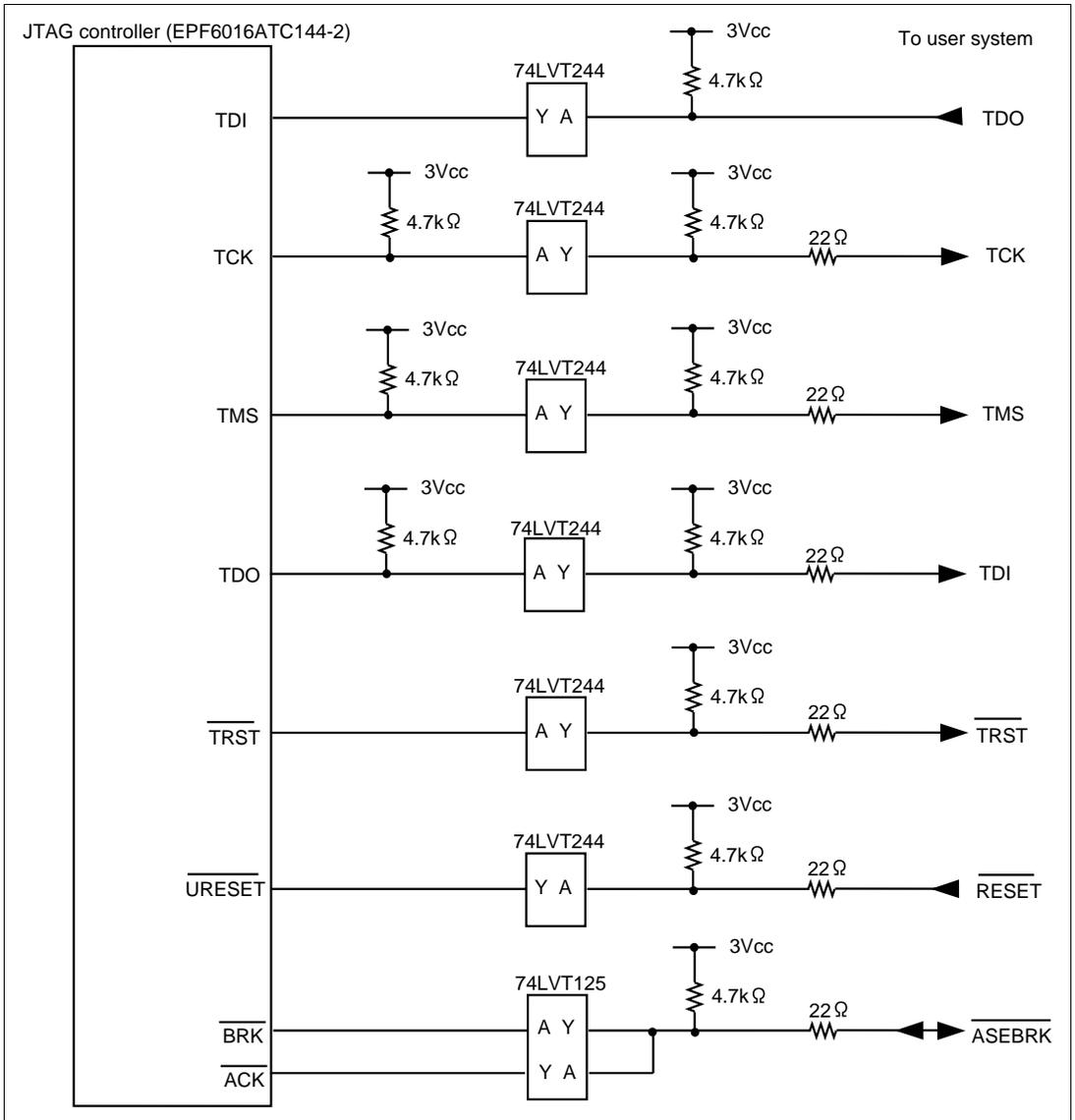
**Figure 6.2 User System Interface Circuit (HS7750RKCM01H)
