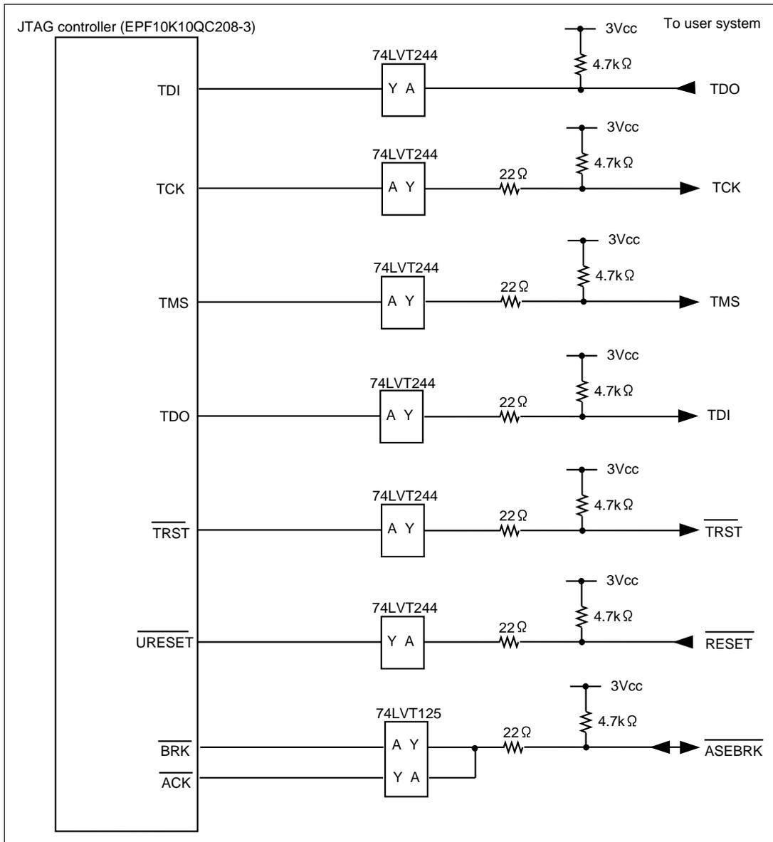
**Figure 6.3 User System Interface Circuit (HS7750RKCI01H)
