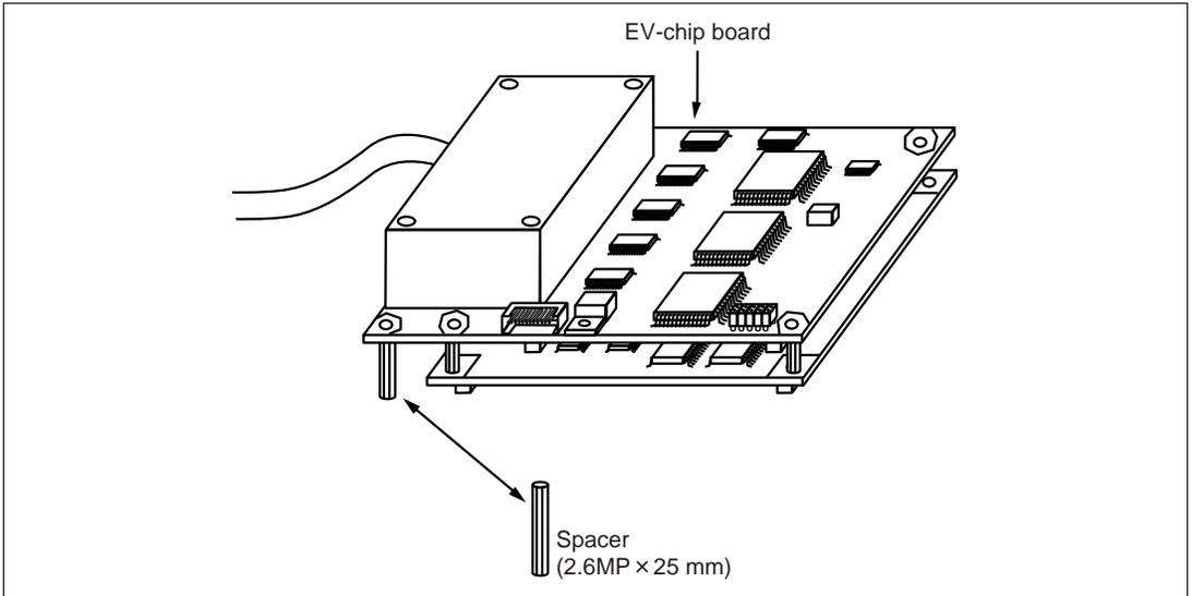
**Figure 4 Exchanging the Spacer**
