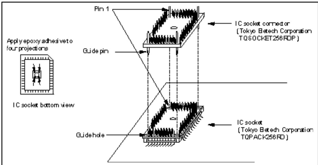
Figure 3 Installing IC Socket to User System
