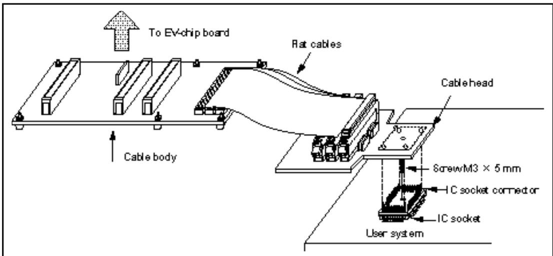
Figure 1 HS 7055ECF81H User System Interface Cable
