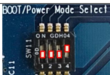
Figure 153: SW11 - QSPI Boot Mode
