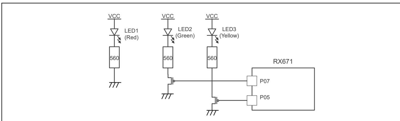
**Figure 2-10. LED Circuit**
