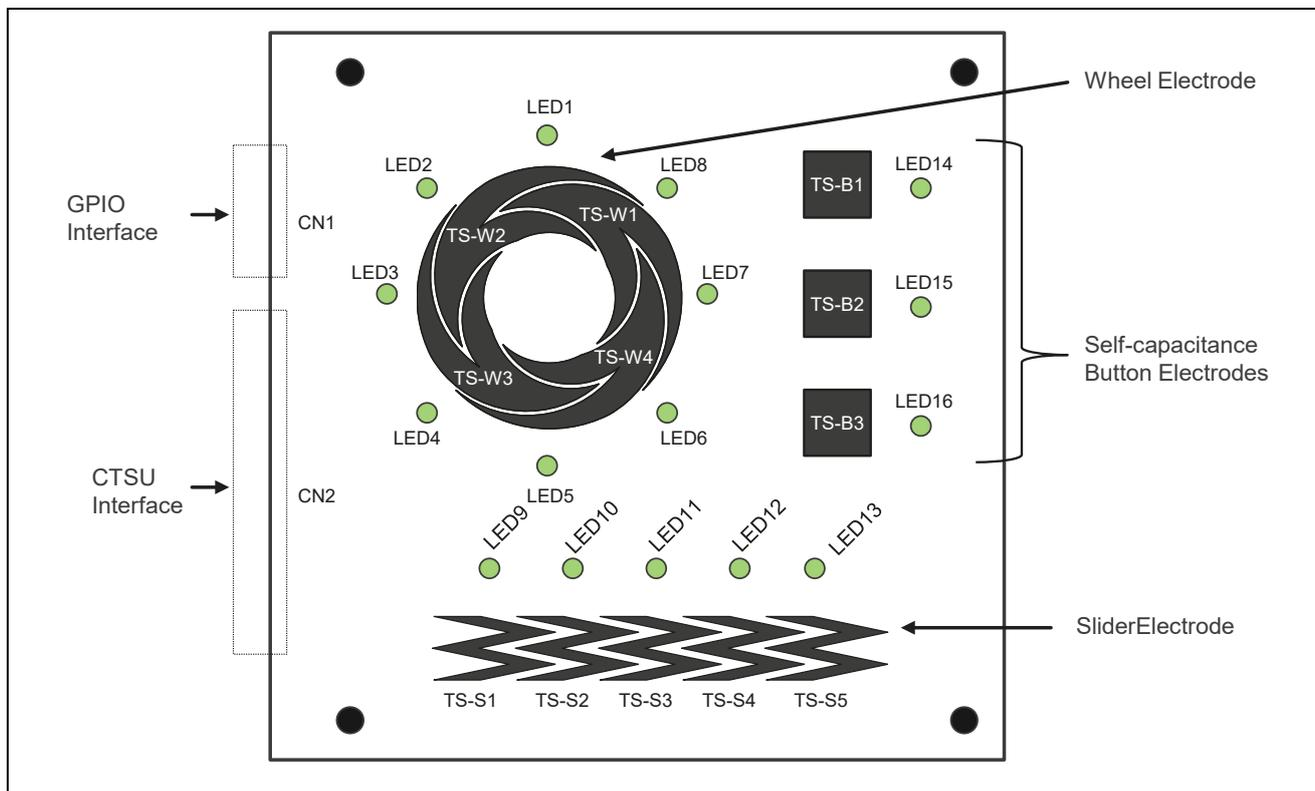
Figure 3-1. Board Layout and TS Pin Assignments
