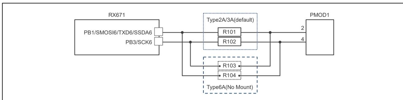
**Figure 2-11. PMOD1 Interface Switch Circuit**
