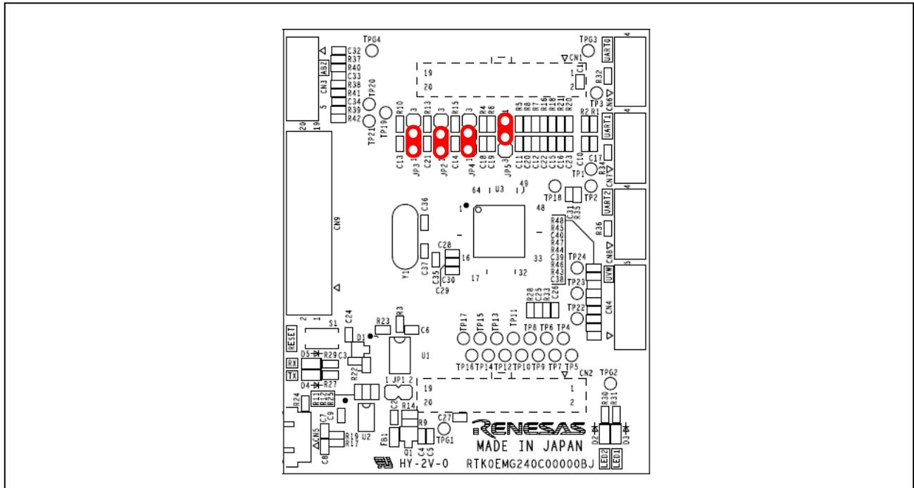
**Figure 8-2 Jumper Pin Assignment on Board - Inverter Board**
