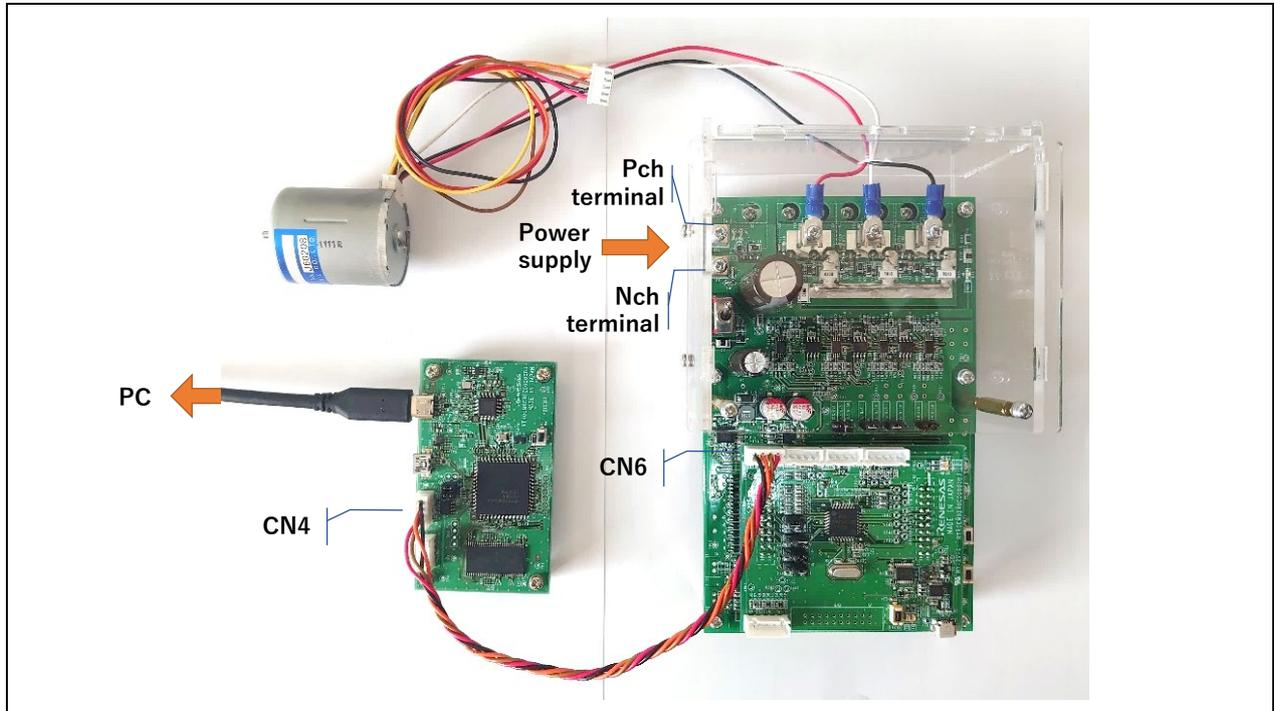
Figure 9-1 Sample Board Connection
