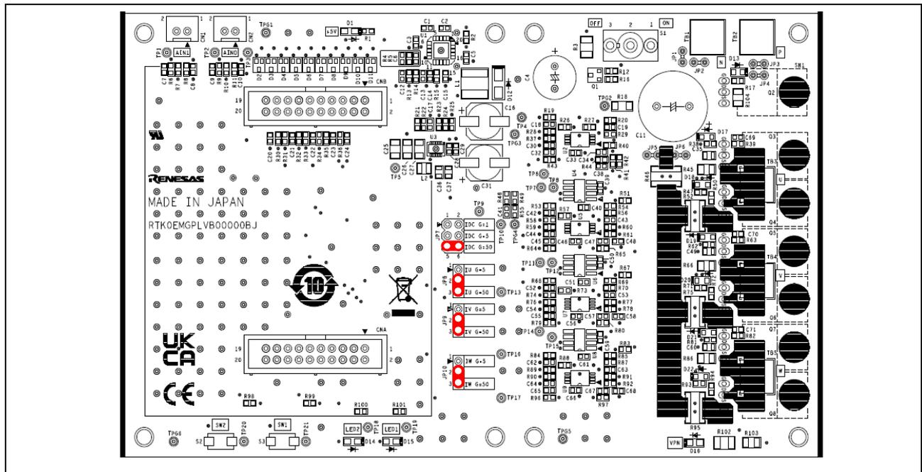
**Figure 8-1 Jumper Pin Assignment on Board - Inverter Board**
