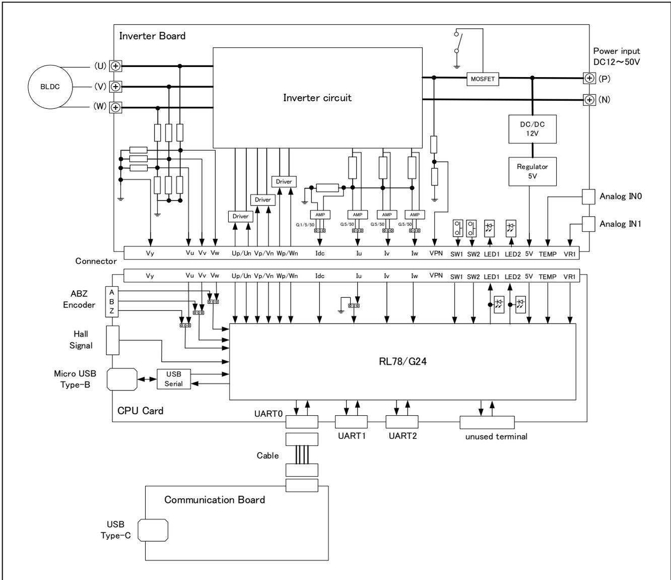
Figure 4-1 Hardware Configuration
