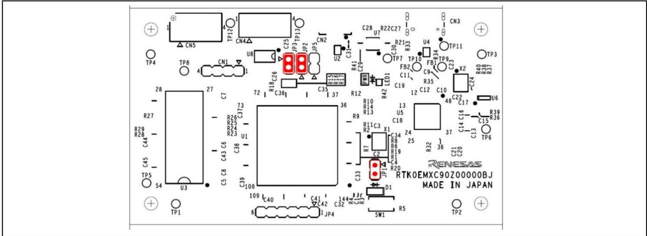
**Figure 8-3 Jumper Pin Assignment on Board – Communication Board**
