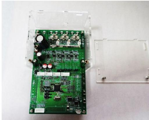
Step 3: Screw in the PMSM cable and power cable. Attach the top panel again.
