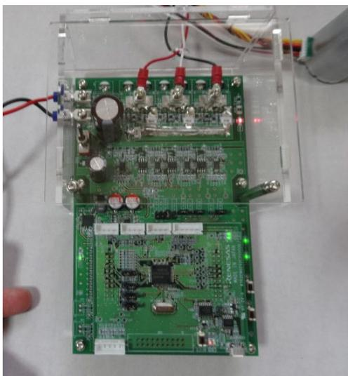
Step 6: Confirm that pressing SW1 drives the PMSM and pressing SW2 stops the PMSM.
