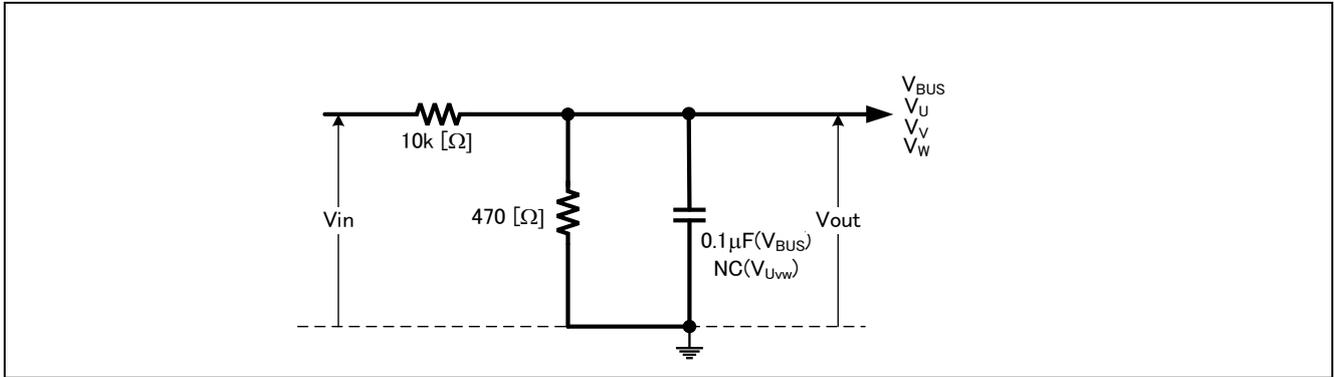
Figure 10-3 Schematic Diagram of Output Voltage Detection Circuit
