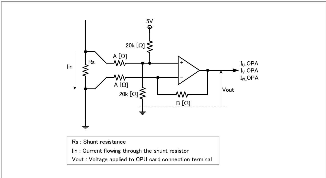
Figure 10-2 Schematic Diagram of Current Detection Circuit
