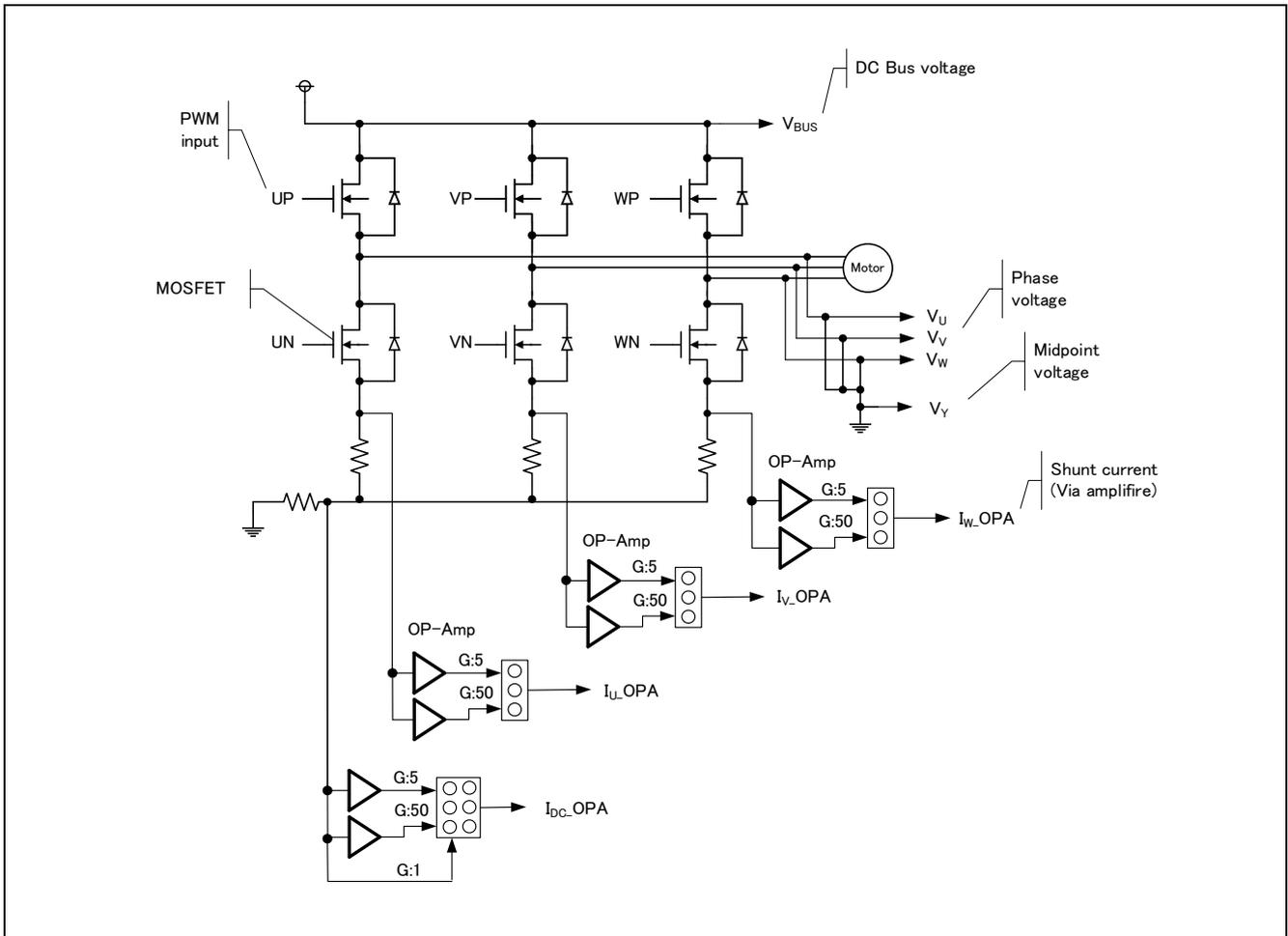
**Figure 10-1 Schematic Diagram of Inverter Control Circuit**
