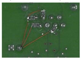
The four missing resistors are soldered on the bottom side of the PCB directly to the related pins of the Ethernet connector and are wired to 3.3V voltage close-by.
