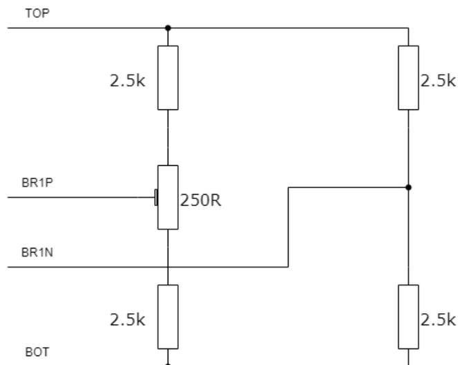
Figure 4: Schematic of the Board Sensor Circuit [4]
