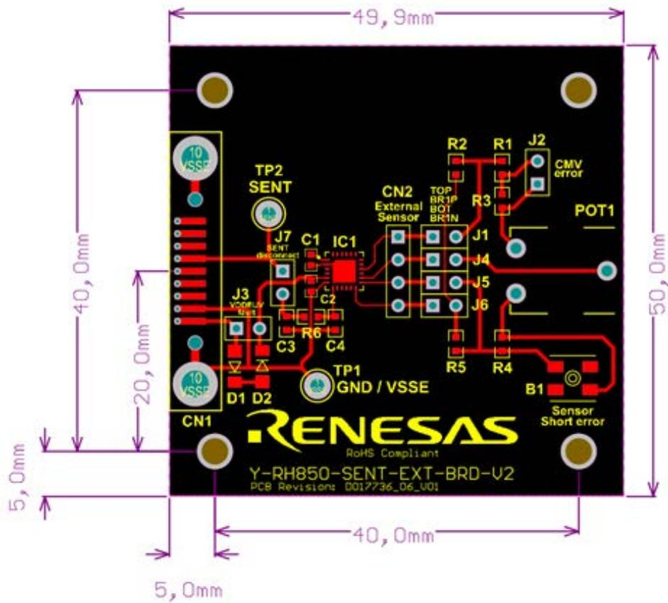
Figure 5: RH850 SENT Application Board dimensions
