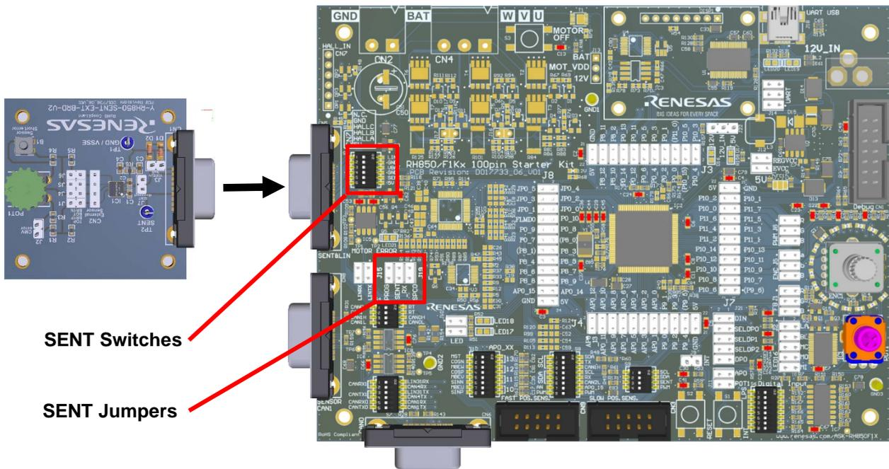
Figure 2: Interconnection with the Y-ASK-RH850F1KM-S1-V3
