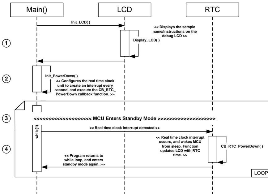
Figure 4-7: Power\_Down Sequence Diagram
