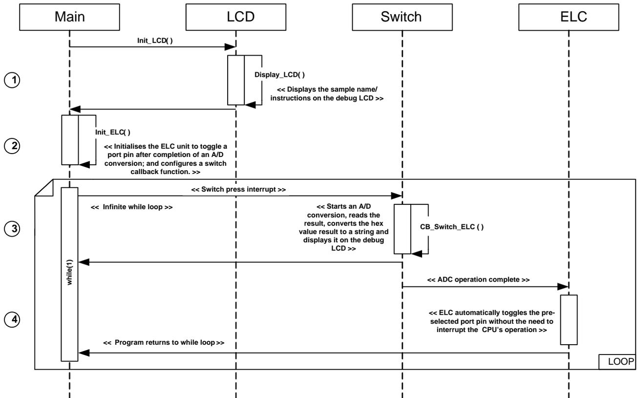
Figure 4-17: Event Link Controller (ELC) Sequence Diagram
