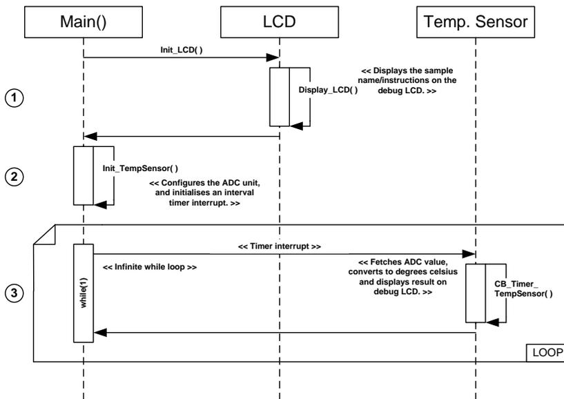
Figure 4-14: Temperature Sensor Sequence Diagram
