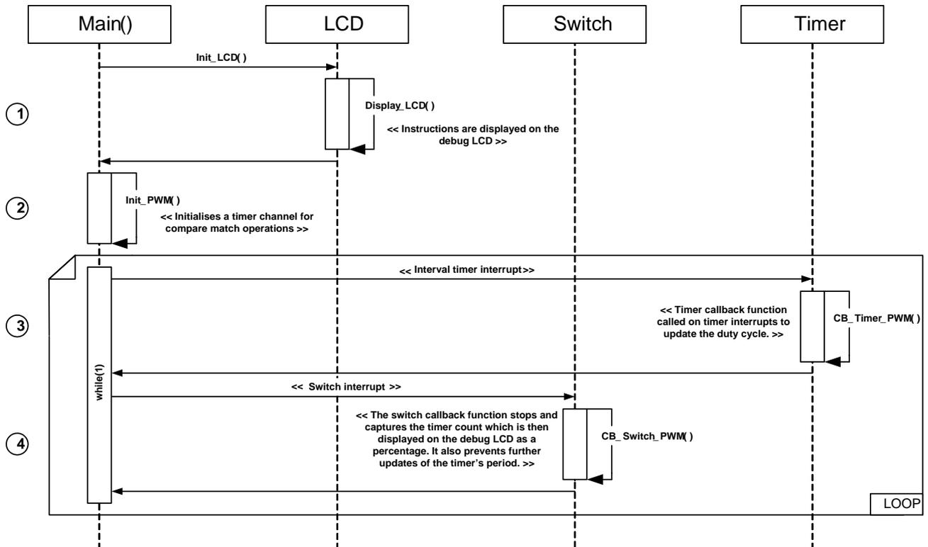
Figure 4-9: PWM Sequence Diagram
