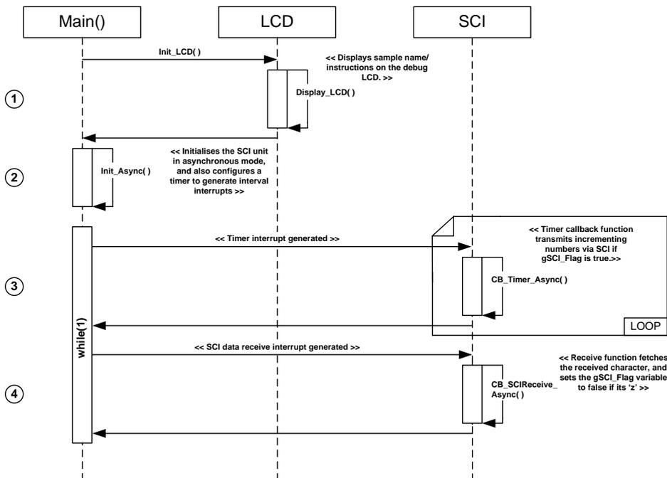
Figure 4-2: Async\_Serial Sequence Diagram
