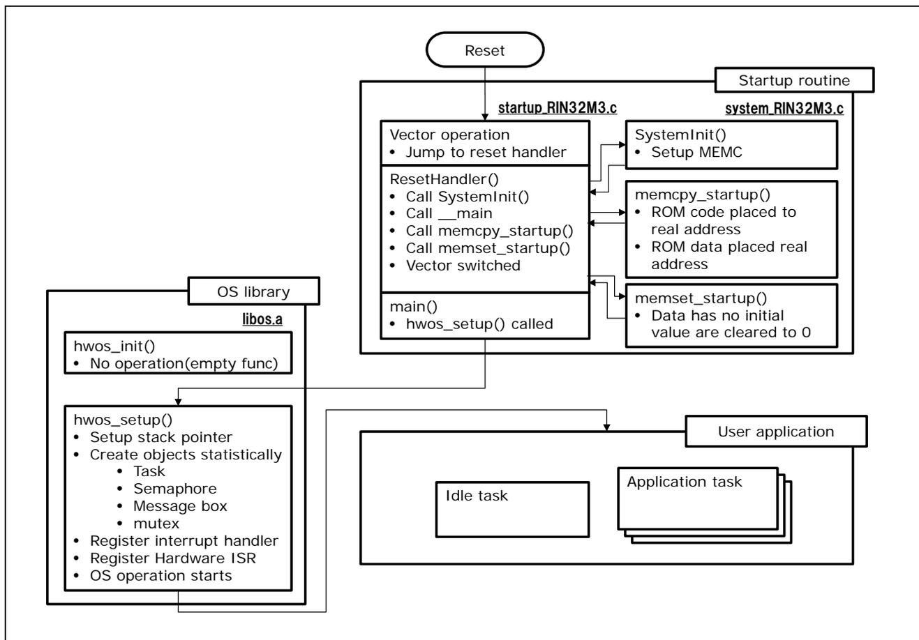
Figure 9.3 Startup Routine with the GNU Compiler
