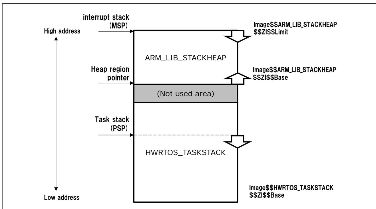
Figure9.2 Stack Area at Startup of the Operating System with the ARM Compiler
