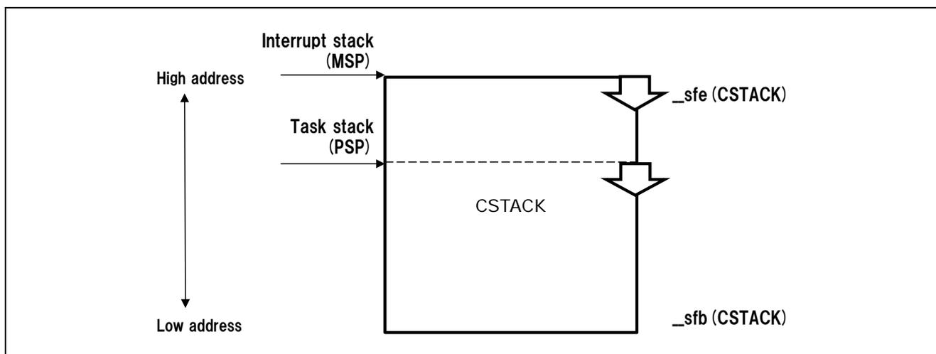
**Figure9.6 Stack Area at Startup of the Operating System of the IAR Compiler**
