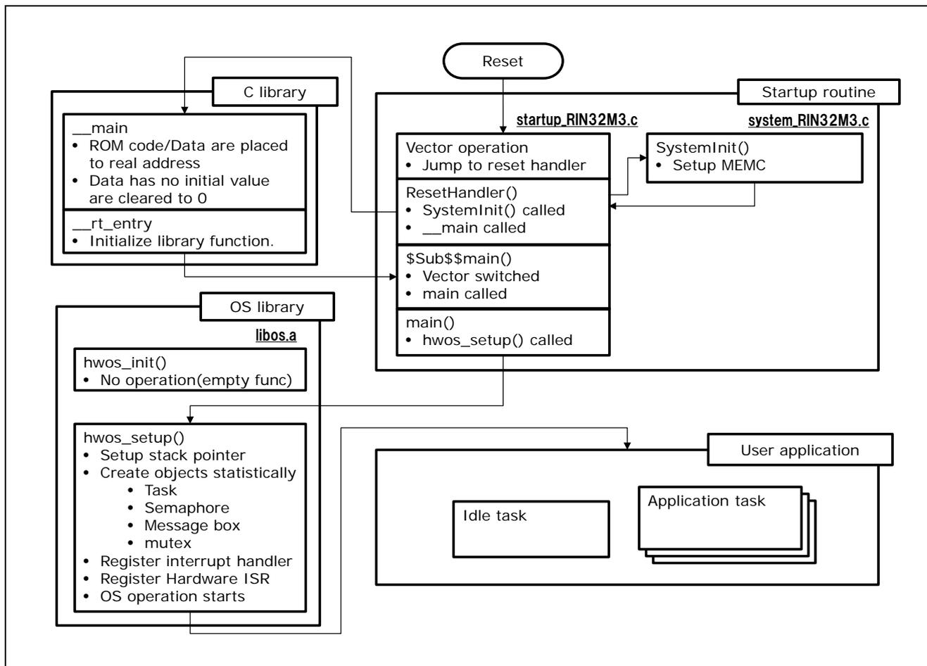
Figure9.1 Startup Routine with the ARM Compiler
