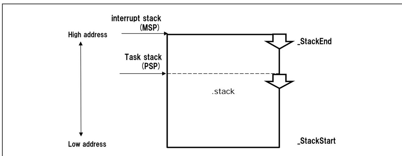
**Figure9.4 Stack Area at Startup of the Operating System with the GNU Compiler**
