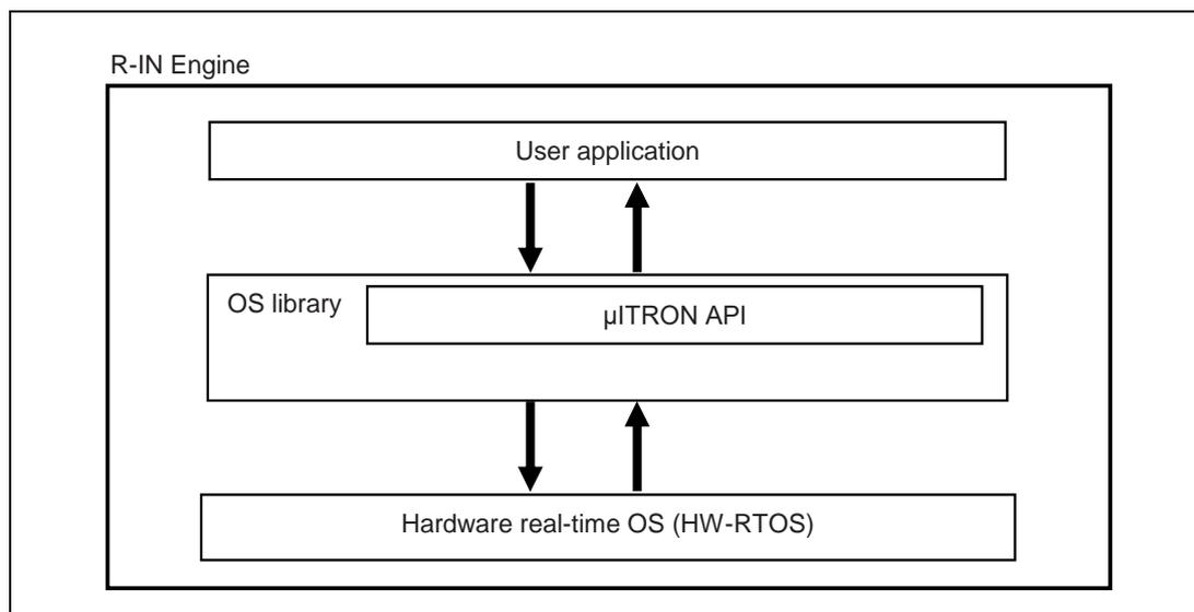
**Figure1.1 System Configuration**
