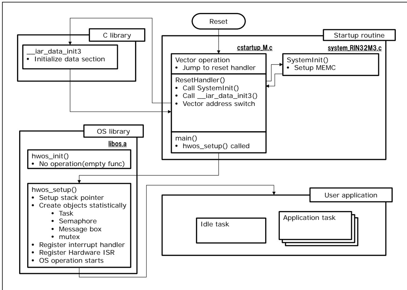
Figure9.5 Startup Routine with the IAR Compiler
