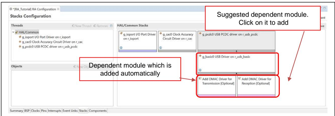
Figure 73. RA Project Configuration – Dependent Module
