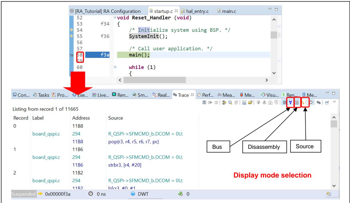
Figure 114. Debug – Select Display Mode In Trace View
