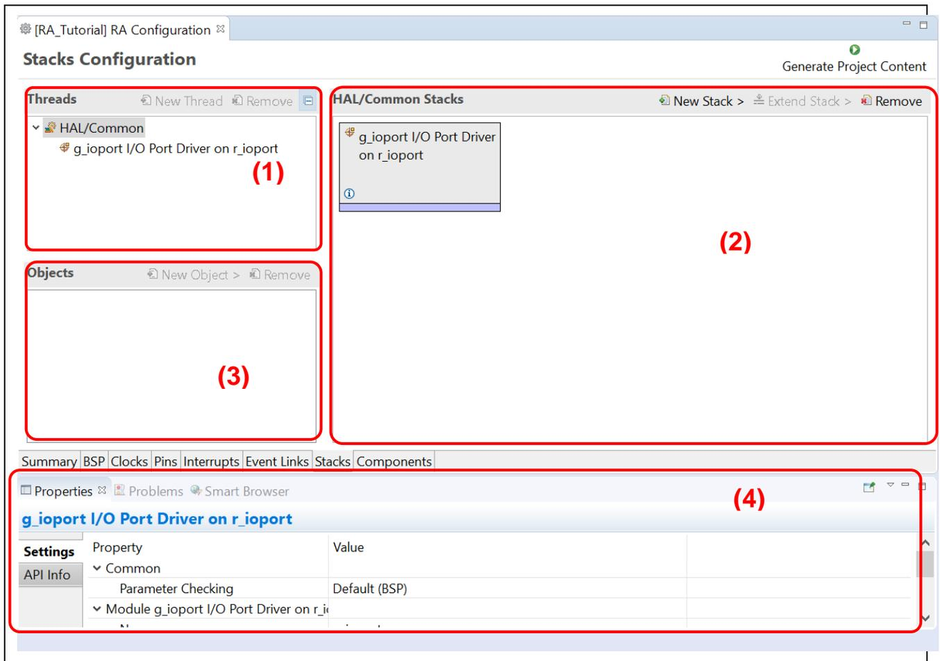
**Figure 71. RA Project Configuration – Stacks Configuration GUI**
