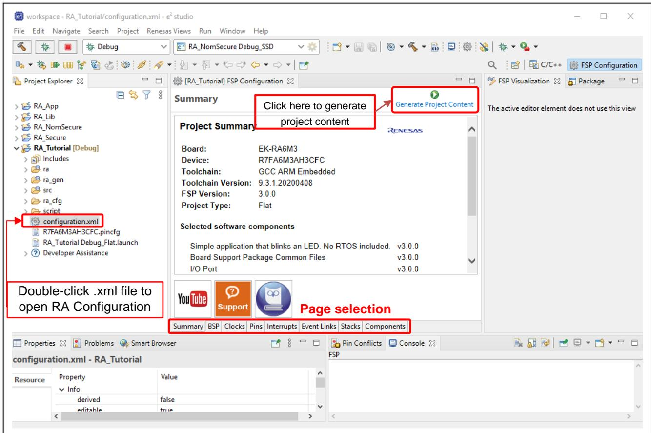
**Figure 58. RA Project Configuration – RA Project Configuration View**
