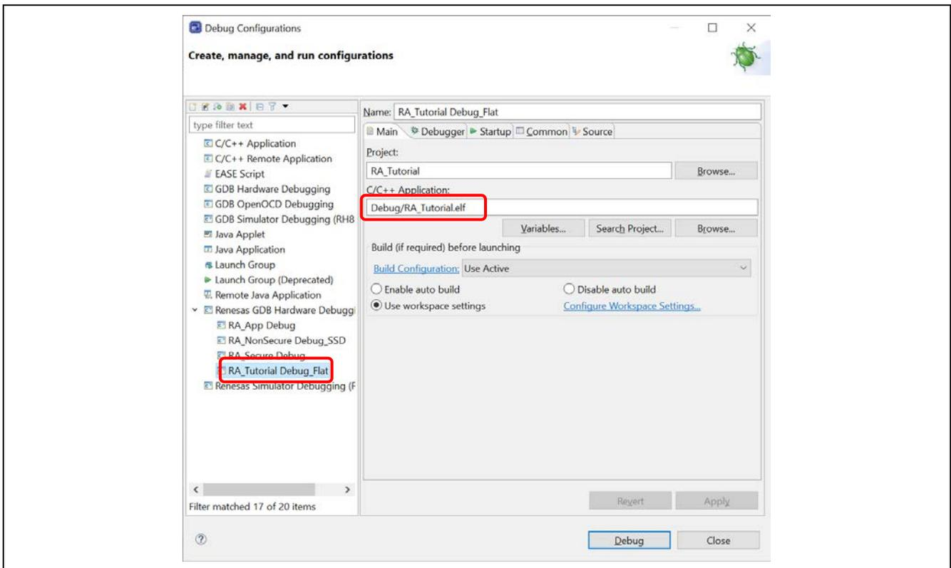
Figure 93. Debug – Selecting the Load Module
