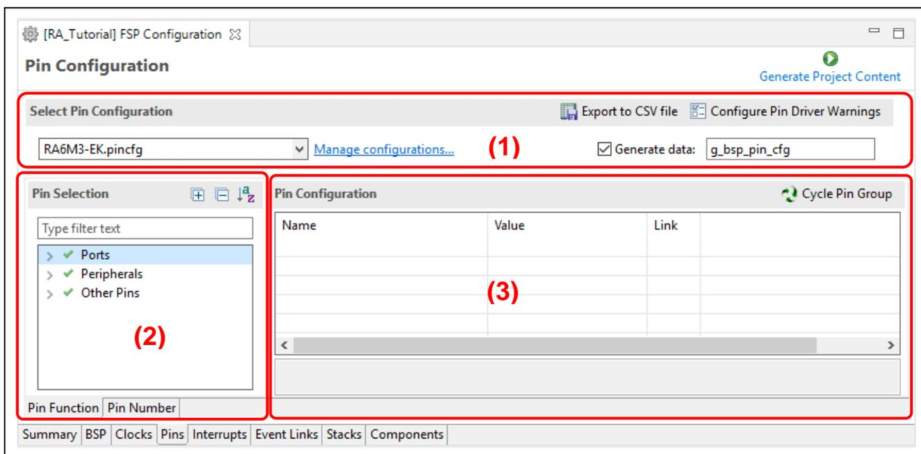
Figure 66. RA Project Configuration – Pin Configuration GUI
