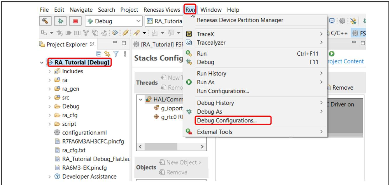
Figure 92. Debug – Opening the Debug Configurations Window
