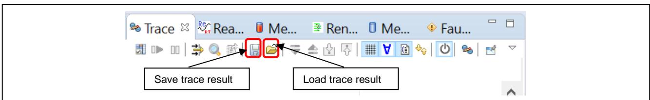
**Figure 117. Debug – Save And Load Trace Result**
