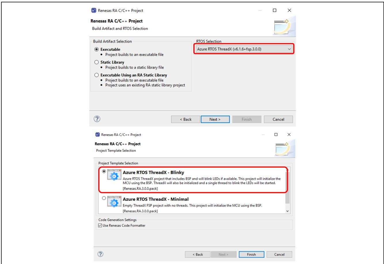
Figure 129. Setting up an Azure RTOS Application - Create New Project
