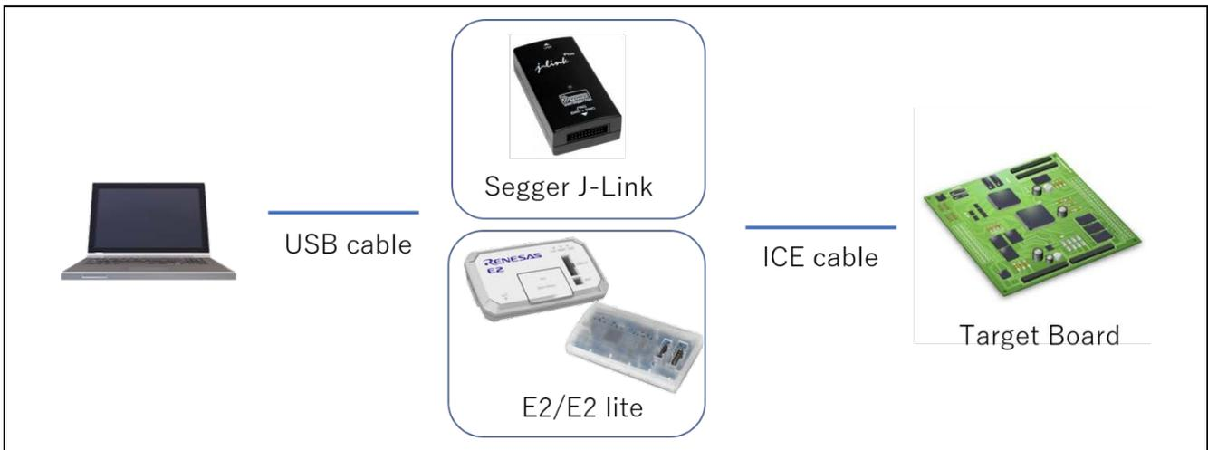
Figure 2. System Configuration
