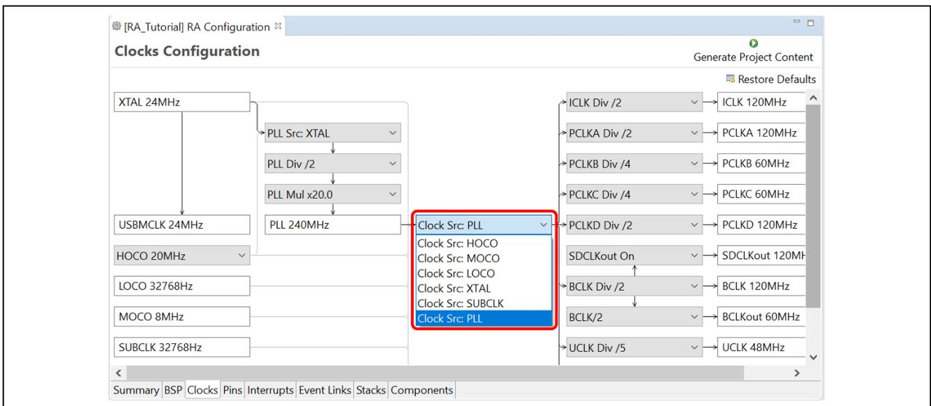
Figure 62. RA Project Configuration – Clocks Configuration
