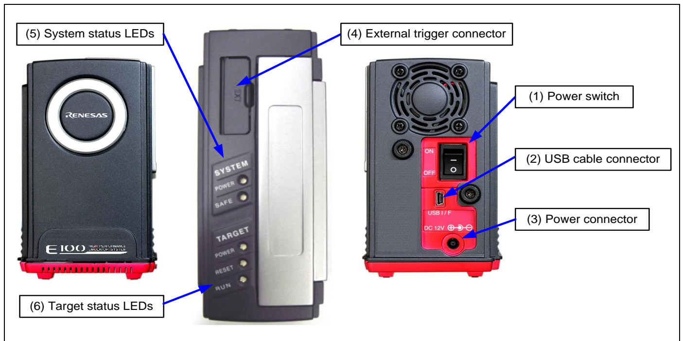
Figure 1.2 Names of the emulator parts
