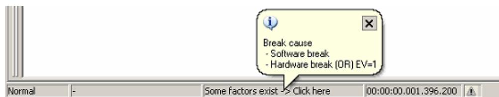
Figure 5.15 Checking the source of a break
