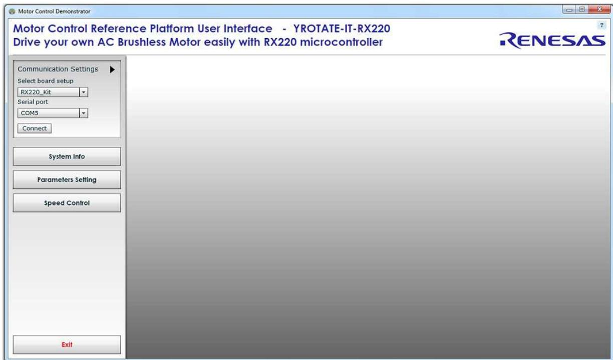
Once connected the GUI can be used to control the motor manually using the **“RPM Control”** facility. Here the user can start, stop and set direction and speed of the motor, whilst observing its performance parameters within the system display windows of the GUI.
