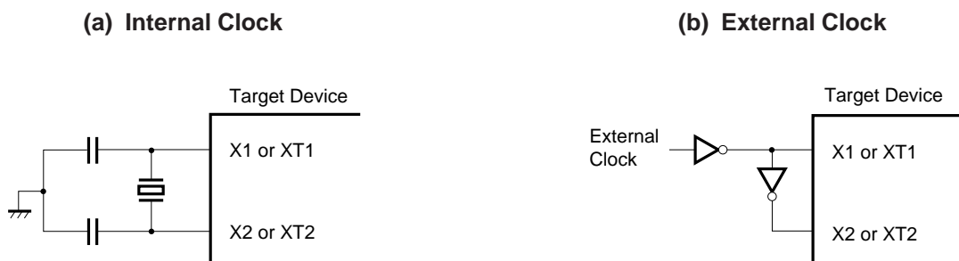
Figure 4-1: System Clock Oscillator External Circuit
