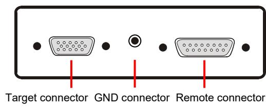
Figure 2.4 FP6 Target Connector Side
