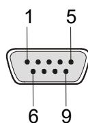
Figure 10.4 Pin Assignments of the Serial Connector
