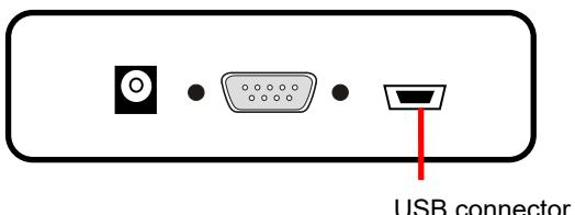
Note: Part number of the mini-B USB connector: UX60SC-MB-5S8 (manufactured by Hirose Electric Co., Ltd.)
