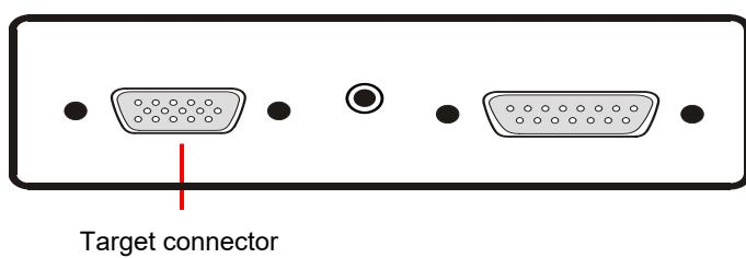
**Figure 10.8 Target Connector (Target Connector Side of the FP6)**
