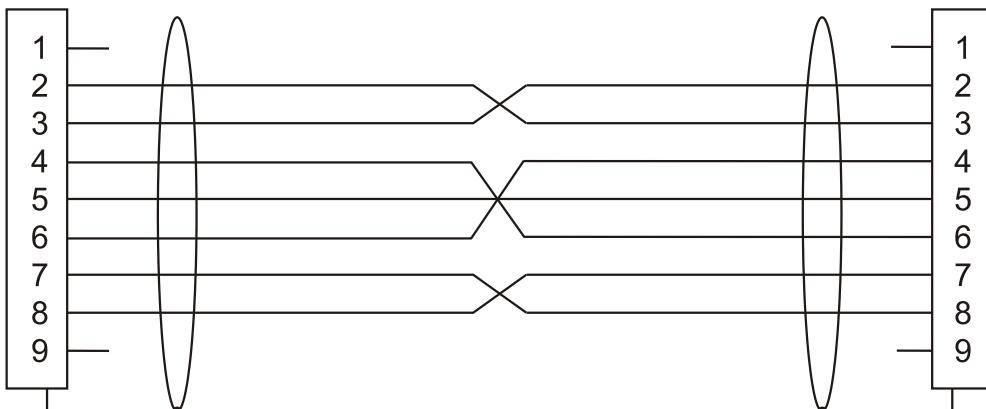
Figure 10.5 Connection of the Serial Cable
