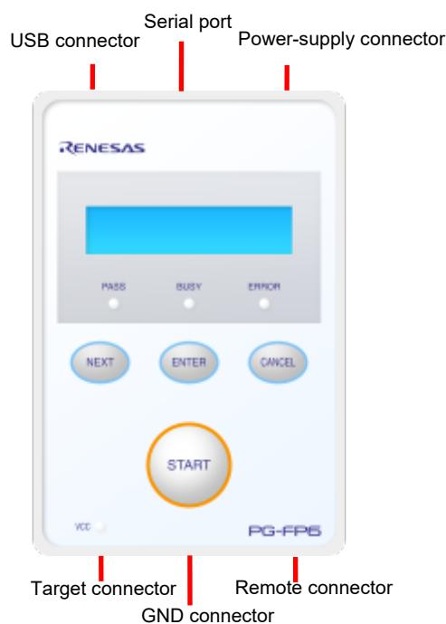
Figure 2.2 FP6 Top View <Connectors>
