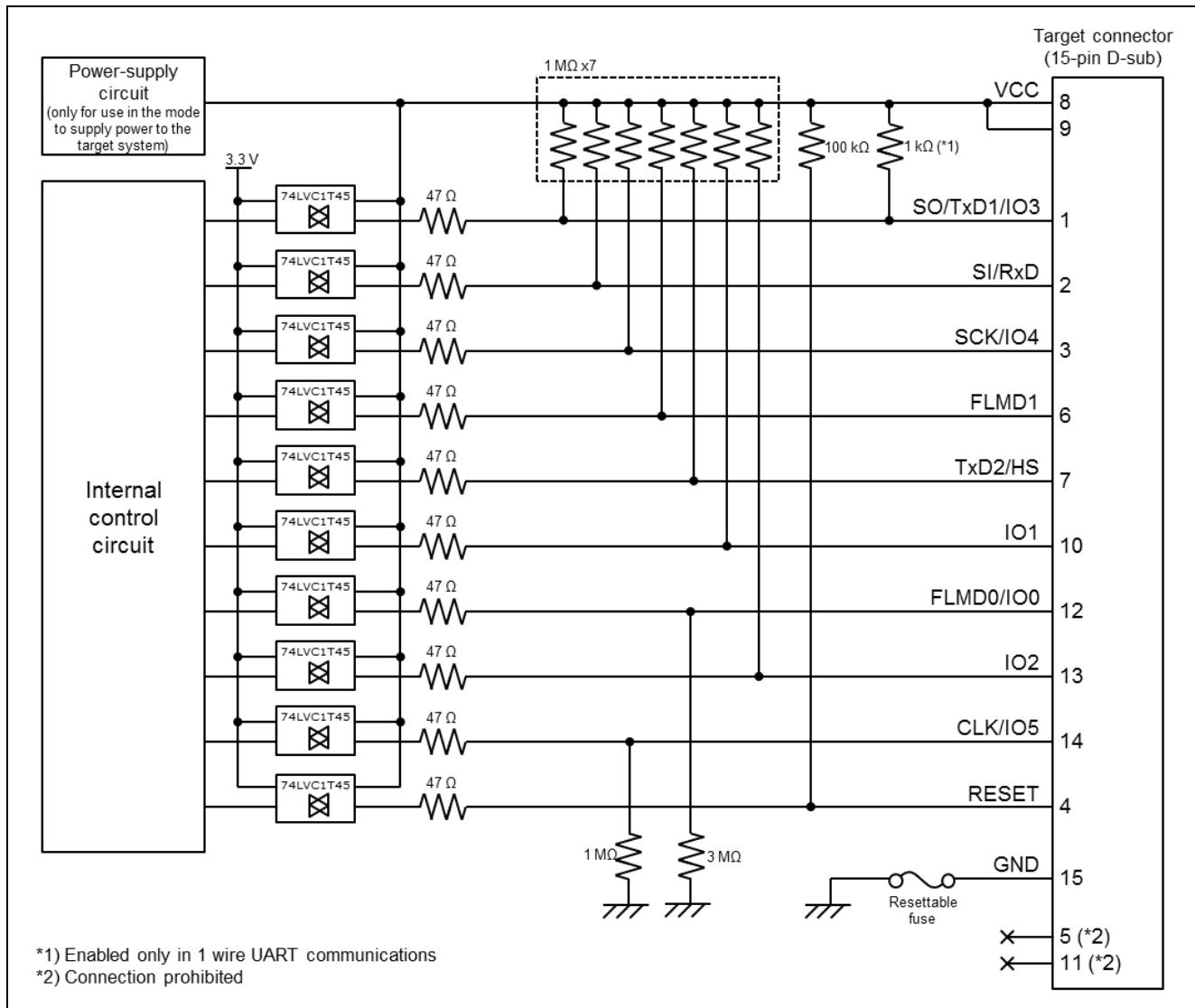
Figure C.1 Equivalent Circuits of the Target Interface
