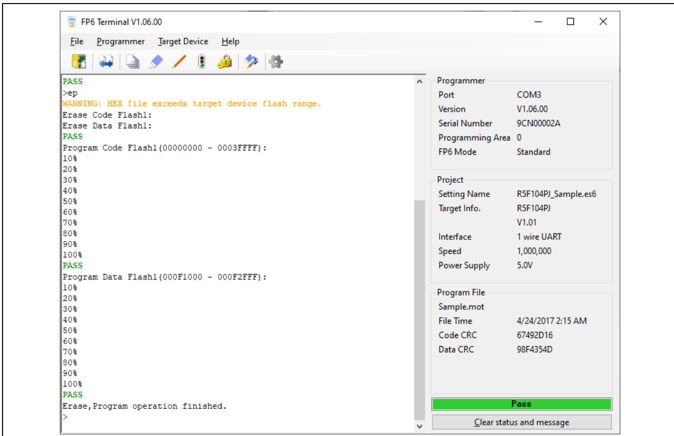
Figure 4.33 Result of Executing the [Start] Command
