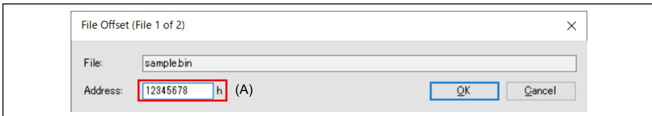
**Figure 4-5 [File Offset] Dialog Box (Address Mode)**
