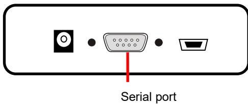
Figure 10.3 9-Pin D-Sub Serial Connector
