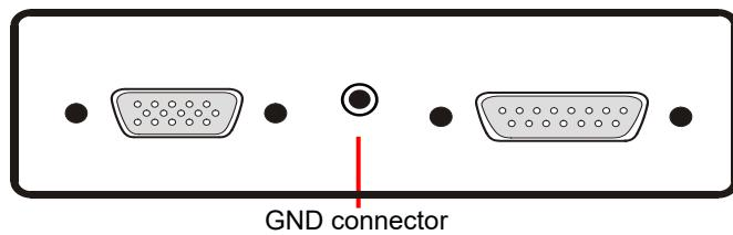
Note: Part number of the GND connector (banana jack): PB4 (manufactured by HIRSCHMANN)
