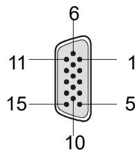
Figure 10.11 Pin Assignments of the 15-Pin D-Sub Male Connector of the Target Cable (14-Pin Type)
