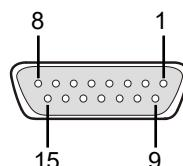
Note: Part number of the remote connector (a 15-pin D-sub female connector): DALC-J15SAF-20L9E (manufactured by Japan Aviation Electronics Industry, Limited)
