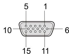
Note: Part number of the target connector (15-pin D-sub female connector): D02-M15SAG-20L9E (manufactured by Japan Aviation Electronics Industry, Limited)
