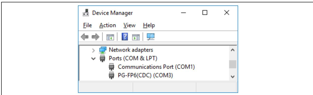
Figure 7.1 Checking the COM Port Number Settings
