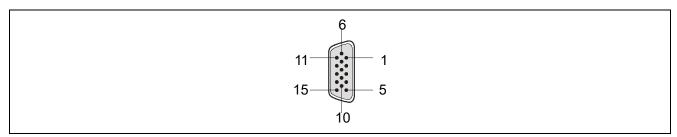
Figure 10.11 Pin Assignments of the 15-Pin D-Sub Male Connector of the Target Cable (14-Pin Type)
