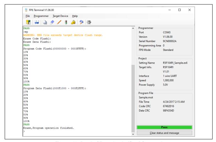
Figure 4.33 Result of Executing the [Start] Command
