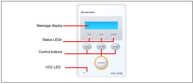
Figure 2.1 FP6 Top View <Control Panel>
