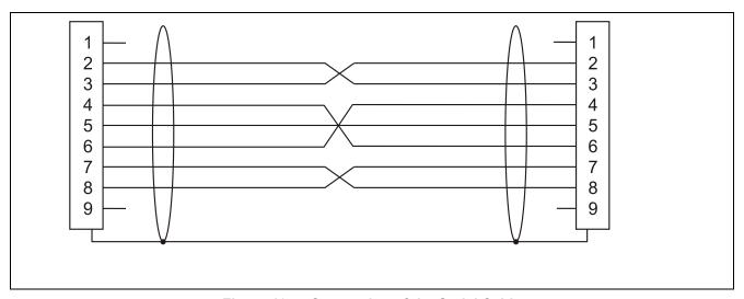
Figure 10.5 Connection of the Serial Cable
