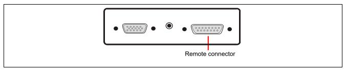
Figure 10.15 Remote Connector (Target Connector Side of the FP6)
