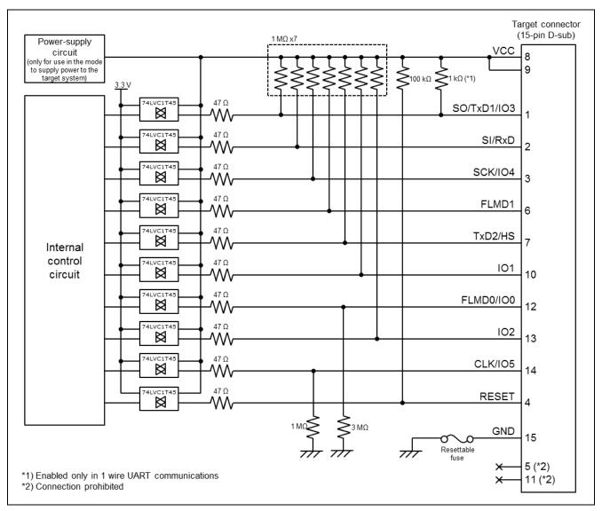
**Equivalent Circuits of the Target Interface** Figure C.1
