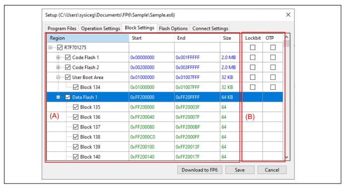
Figure 4.9 [Block Settings] Tabbed Page (Case of Other Device Types)
