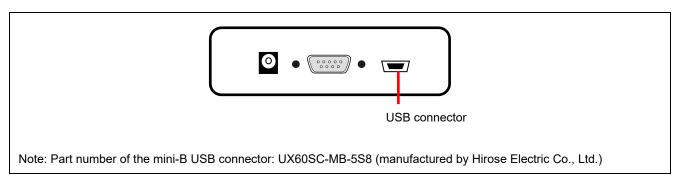
Figure 10.6 USB Connector (Host Interface Side of the FP6)
