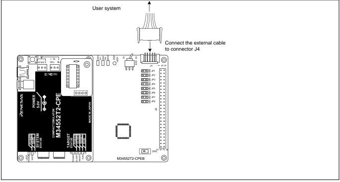
Figure 2.18 Connecting the external trace/trigger cable
