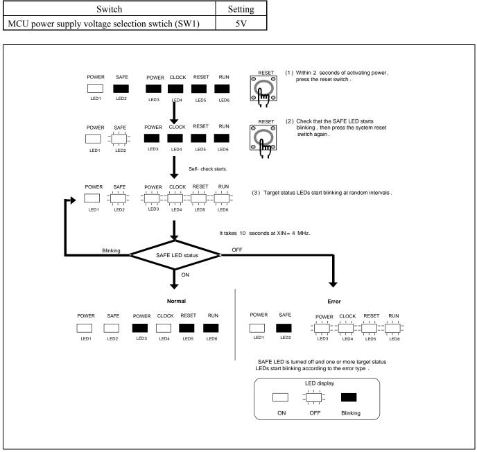
Figure 2.9 Self-check procedure
