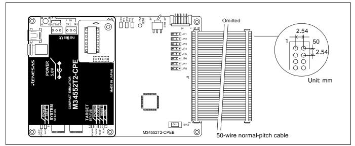
Figure 2.11 Connecting to a 50-pin 2.54-mm-pitch user system
