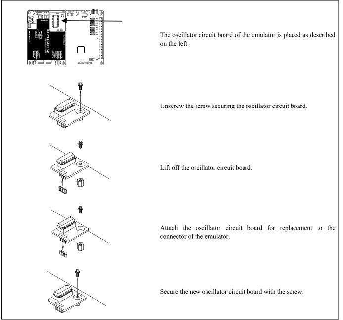
Figure 2.15 Replacing oscillator circuit boards
