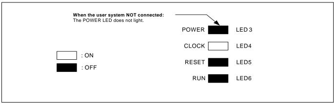
Figure 2.7 Target status LEDs display when the emulator starts up normally (when user system not connected)
