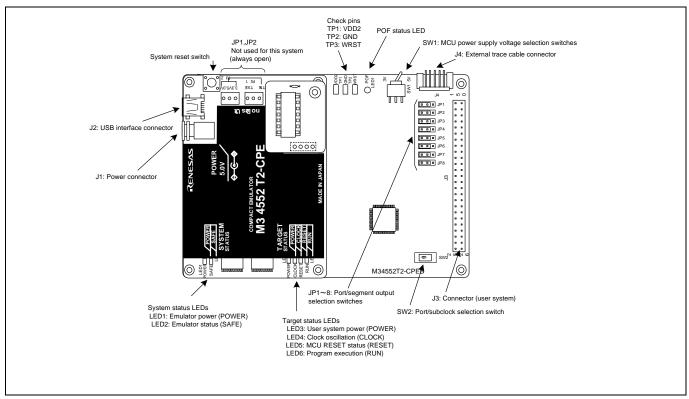
Figure 1.2 Names of the LEDs on the upper panel of the M34552T2-CPE
