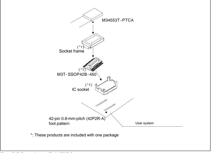
Figure 2.12 Connecting to a 42-pin SSOP foot pattern
