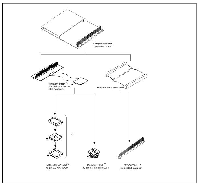
Figure 2.10 Connection of the M34552T2-CPE and user system
