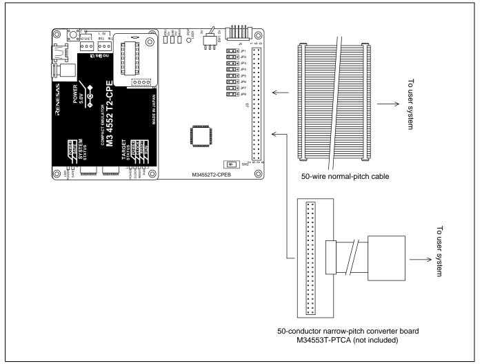
Figure 2.13 Connecting to the M34553T-PTCA
