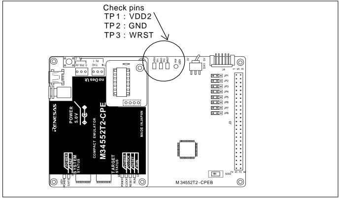
Figure 2.22 Positions of the check pins
