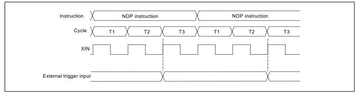
Figure 2.21 Latch timing of external trace input
