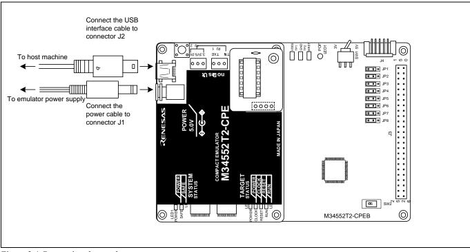
Figure 2.4 Connecting the emulator system
