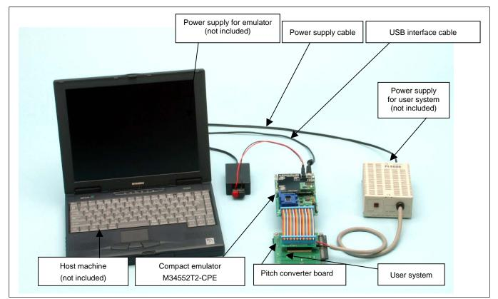
Figure 1.1 System configuration
