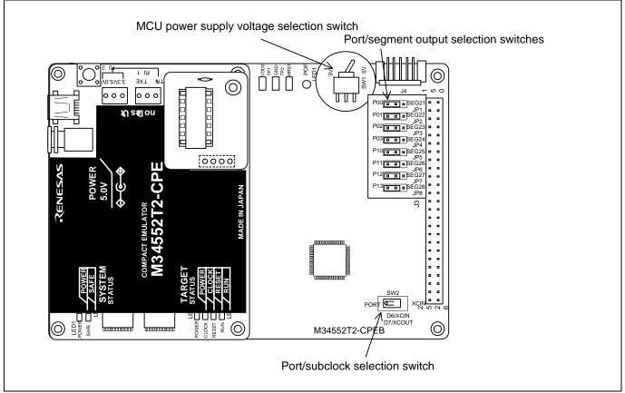
Figure 2.5 Jumper switch locations of the emulator
