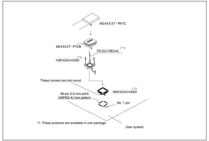
Figure 2.14 Connecting to the 48-pin 0.5-mm-pitch LQFP package foot pattern
