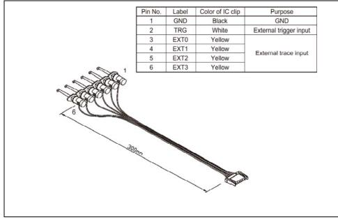
Figure 2.19 Pin assignment of the external trace cable
