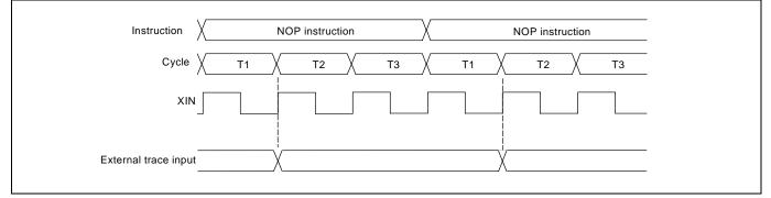
Figure 2.20 Latch timing of external trace input
