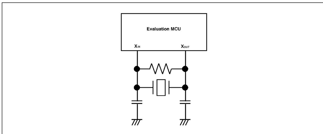
Figure 2.26 Circuit in which oscillation does not occur
