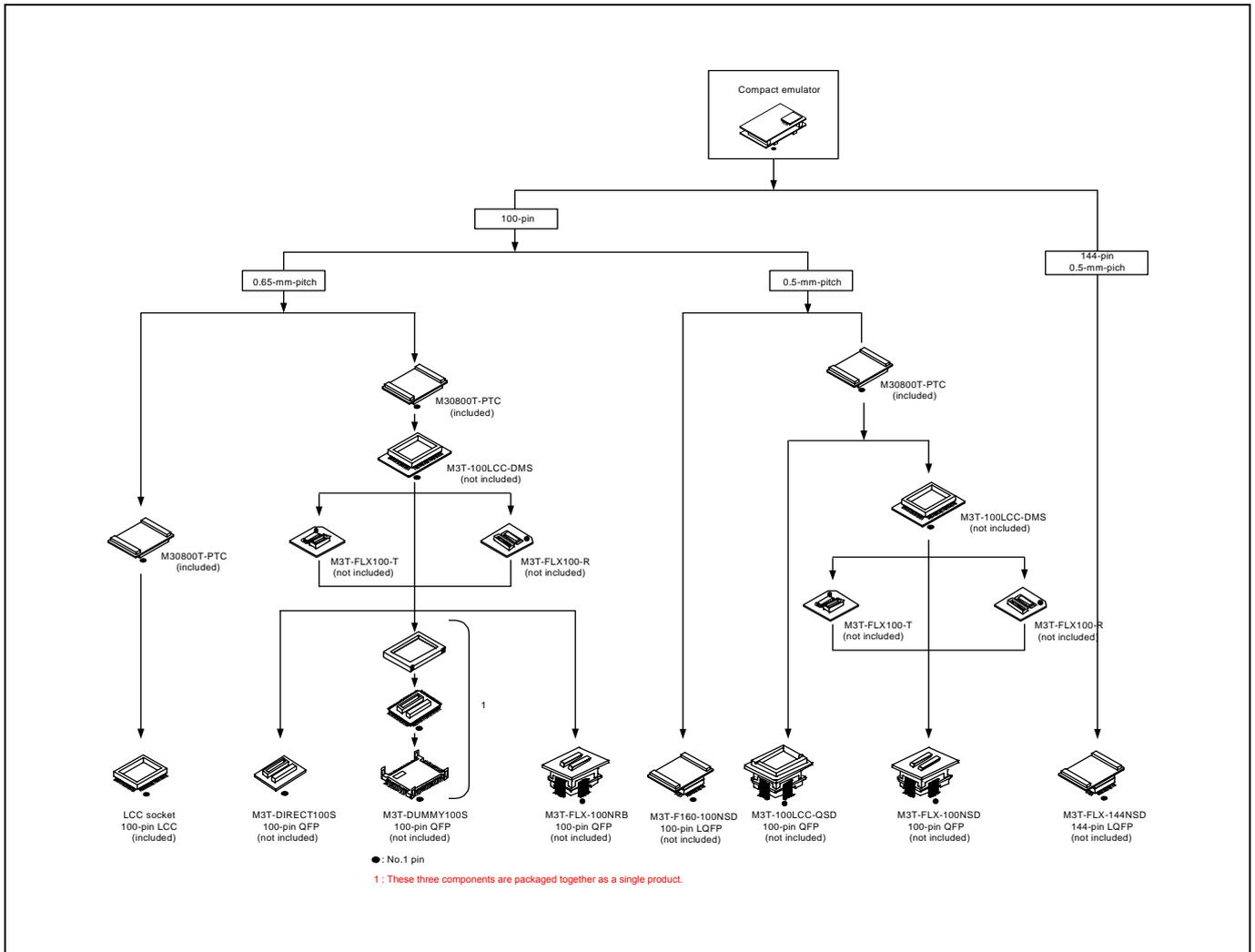
Figure 2.11 Connection of the M30870T2-CPE and user system
