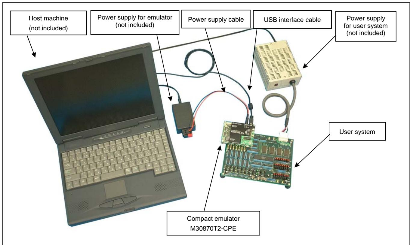
Figure 1.1 System configuration
