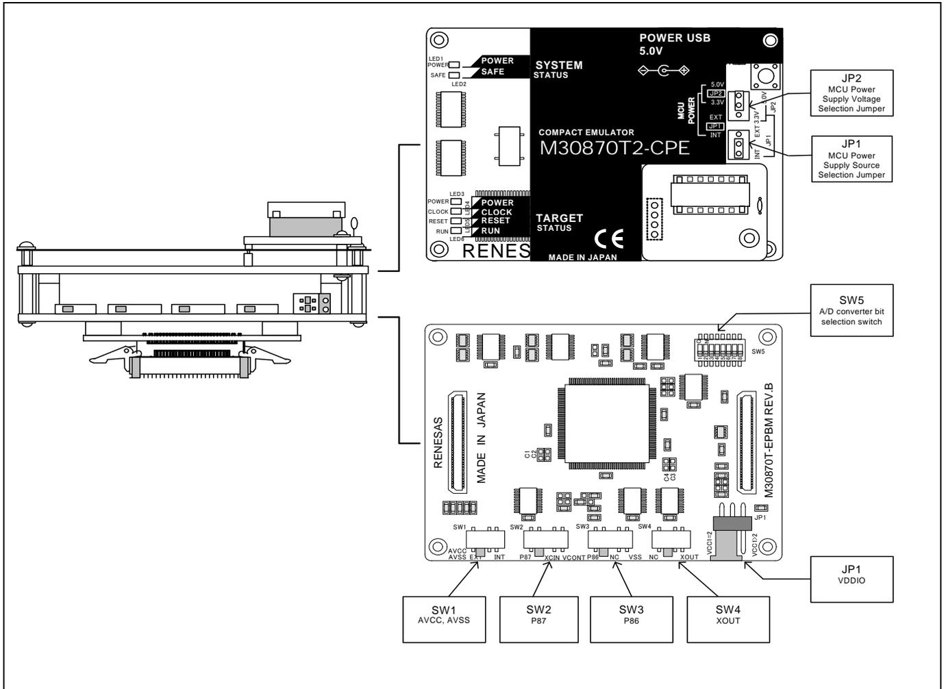
Figure 2.20 Positions of the switches (with M30870T-EPBM REV.B)
