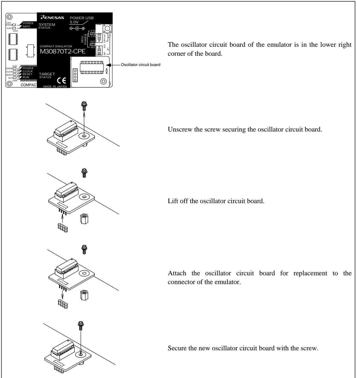
Figure 2.22 Replacing oscillator circuit boards
