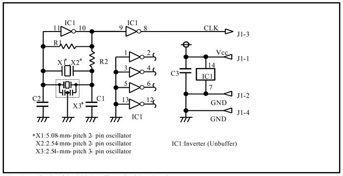
Figure 2.21 Circuits of the OSC-2 oscillator circuit bare board
