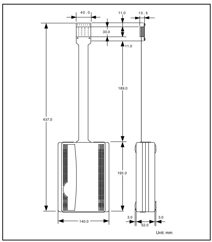
Figure 4.8 External dimensions of the emulation pod
