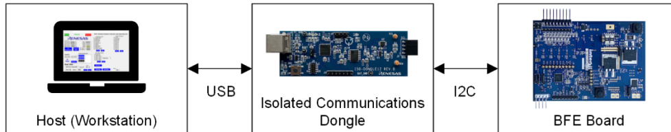
Figure 1. GUI, Communications Dongle and Battery Front End Connection
