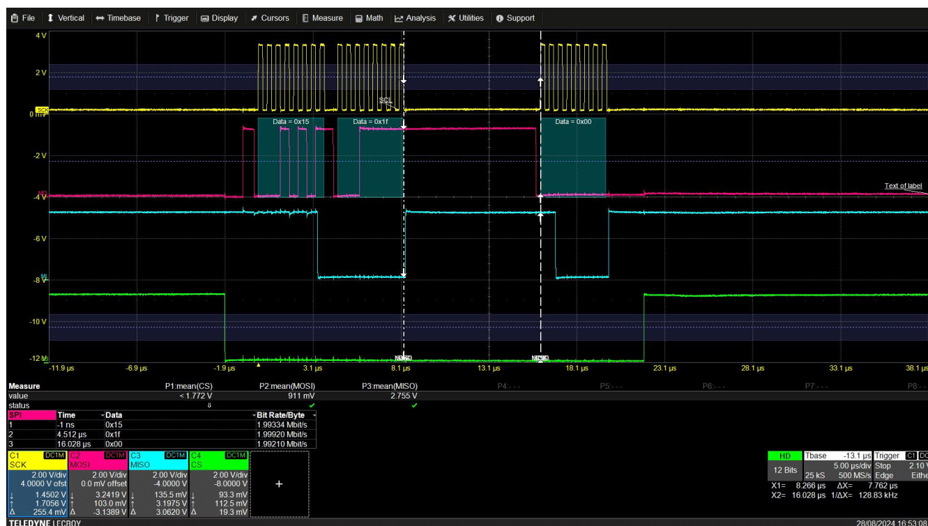
Figure 29. Inter-byte Timing of the SPI Read Command
