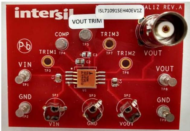
**FIGURE 6. VOLTAGE REFERENCE EVALUATION BOARD (FRONT)**
