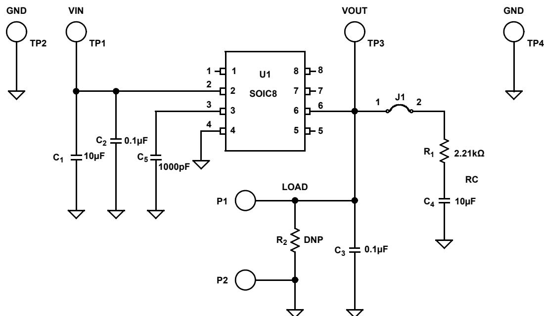
Figure 4. ISL71010BM50EV1Z Evaluation Board Schematic
