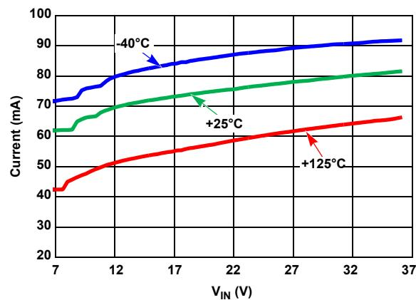
Figure 18. Short-Circuit to  $V_{IN}$
