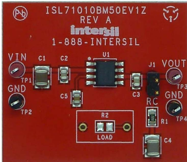
Figure 3. ISL71010BM50EV1Z Evaluation Board
