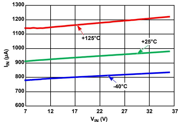
Figure 14.  $I_{IN}$  vs  $V_{IN}$ , Three Temperatures
