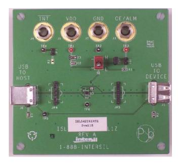
FIGURE 1. ISL54226IRTZEVAL1Z EVALUATION BOARD
