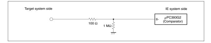
Figure 4-7. Equivalent Circuit G
