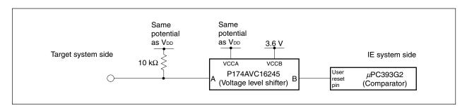
Figure 4-5. Equivalent Circuit E
