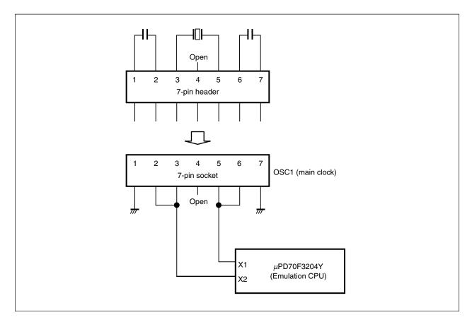
The frequency of the subclock is fixed to 32.768 kHz, so the resonator for the subclock cannot be replaced. The IE-703204-G1-EM1 does not support clock oscillation by the resonator on the target system. Therefore, operation between the resonator on the target system and the oscillator in the target device cannot be emulated using the IE-703204-G1-EM1.
