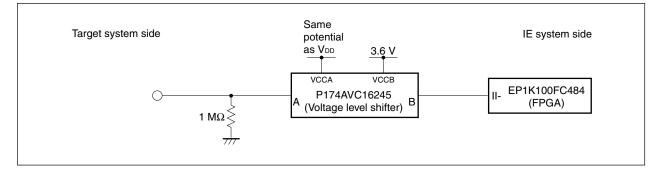
Figure 4-9. Equivalent Circuit I
